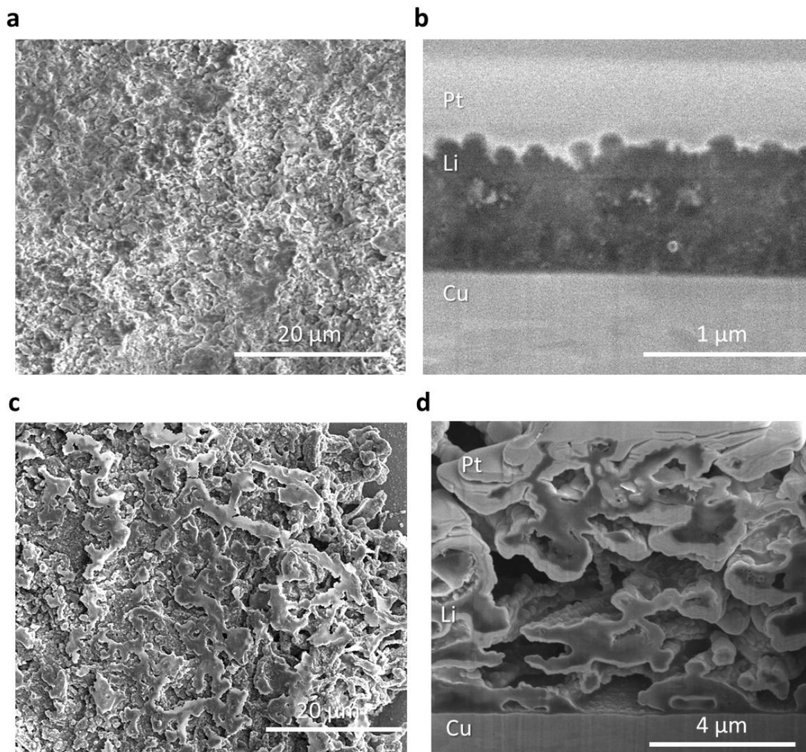
**Figure S6.** Cross-sectional analysis of lithium deposition on current collectors. (a) Top view and (b) side view of the hole-cylinder Au patterned anode after lithiation. (c) top view and (d) side view of the bare Cu electrode after lithiation.
