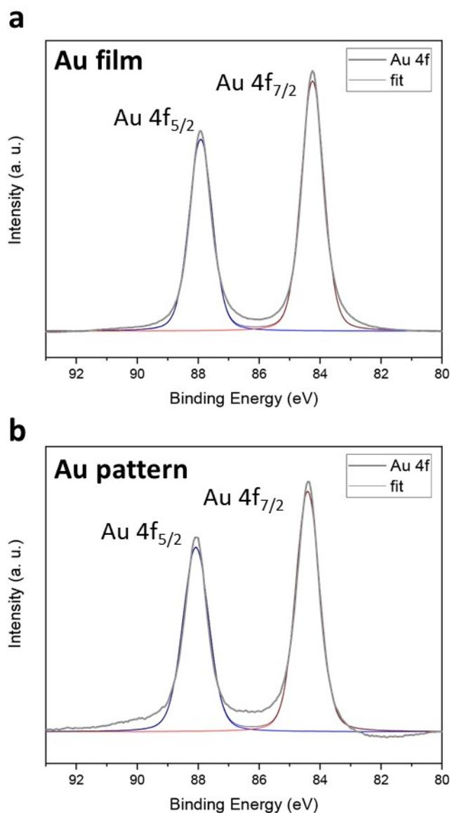
**Figure S4.** X-ray photoelectron spectroscopy (XPS) spectra confirming the metallic state of Au 4f. (a) Au film deposited on Cu current collector and (b) the 3D Au hole-cylinder nanopattern on Cu current collector. In both cases the Au 4f<sub>7/2</sub> and Au 4f<sub>5/2</sub> peaks appear at ~84.0 eV and ~87.7 eV, respectively, with no detectable higher-binding-energy shoulders, indicating that Au remains predominantly in the metallic (Au<sup>0</sup>) state with negligible oxidation.
