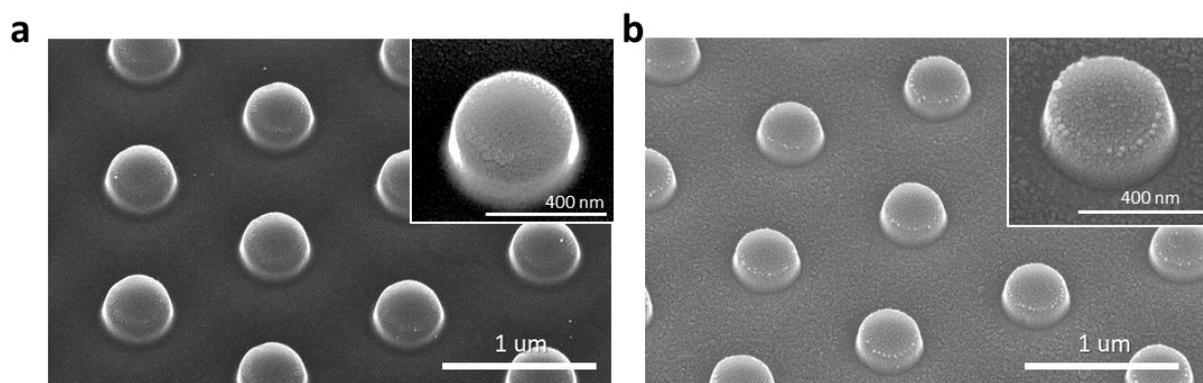
**Figure S1.** Scanning Electron Microscope (SEM) images of polystyrene (PS) prepatterns directly formed on Cu foil. (a) PS prepatterns after nanoimprint lithography, showing the uniform pattern formation on the substrate; (b) PS patterns after the removal of residual PS using reactive ion etching (RIE), illustrating a clean and well-defined pattern on the Cu foil.
