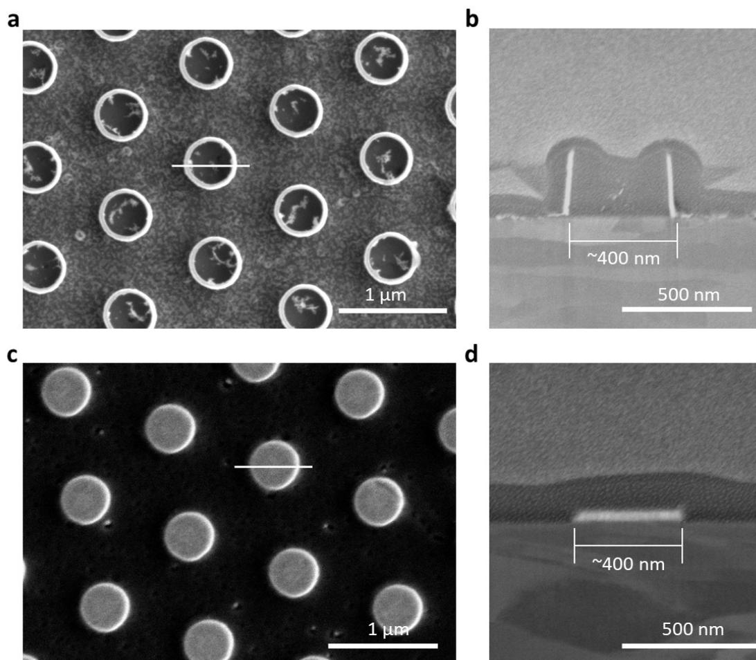
**Figure S5.** Cross-sectional analysis of Au nanopatterns on Cu foil. (a) Top view and (b) side view of the hole-cylinder Au patterned Cu current collector. (c) top view and (d) side view of the flat disk shaped Au patterned Cu current collector. The white line in (a, c) indicates the position of the cross-section.
