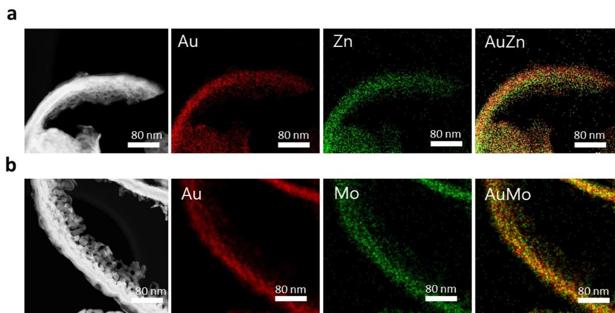
**Figure S8.** EDS mapping of the multi-metal compositions in the fabricated patterns. (a) uniform distribution of Au and Zn within the hole-cylinder pattern. (b) Distribution of Au and Mo within the pattern. The results confirm the effective mixing of metals achieved through secondary sputtering during the  $\text{Ar}^+$  ion bombardment step.
