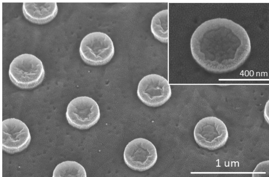
**Figure S2.** SEM images of disk-shaped Au patterns formed after  $\text{Ar}^+$  ion bombardment. The exposed Au regions were etched away, leaving the Au beneath the PS prepatterns intact, resulting in well-defined disk-shaped structures
