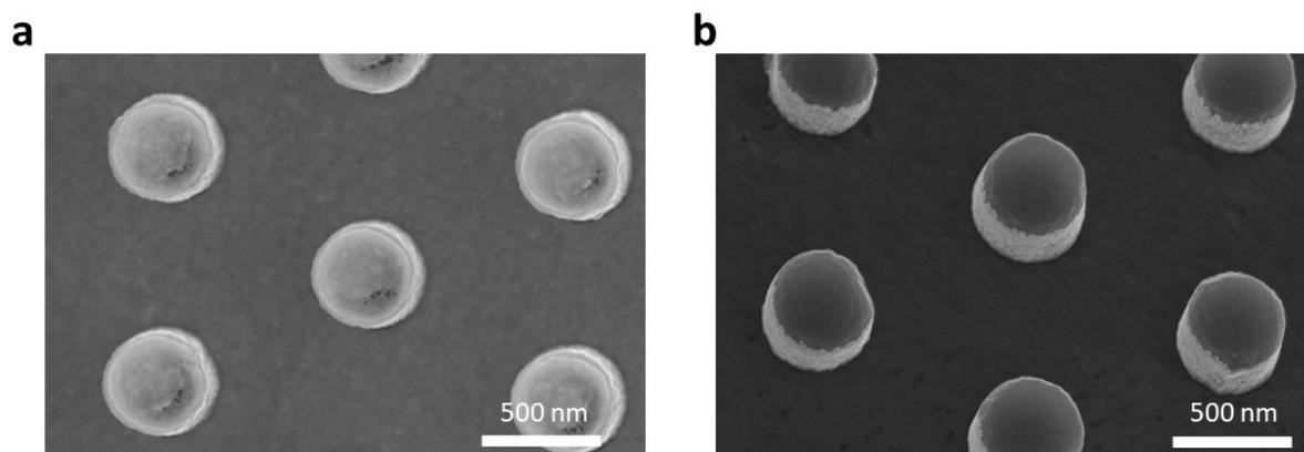
**Figure S3.** SEM images illustrating the fabrication process of hole-cylinder Au patterns. (a) Au deposition onto PS prepatterns. (b) Formation of hole-cylinder Au patterns following  $\text{Ar}^+$  ion bombardment, with the Au conformally attached to the prepattern.
