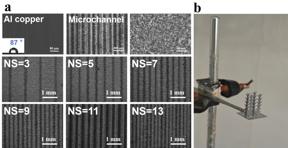
Figure. S2. (a) Schematic diagram of the surface morphology before and after the etched graded microchannels on the surface of aluminum sheet and the surface structure of the microchannels of different orders. (b) The optical image of the SHBS@BIS array fog collector.
