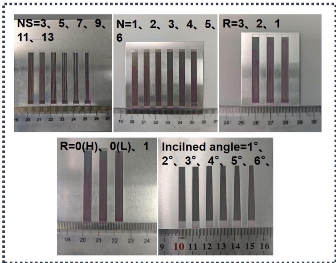
Figure. S3. Microchannel width NS, groove depth H, low: high order quantity ratio R and the influence of inclined angle on liquid transport distance.
