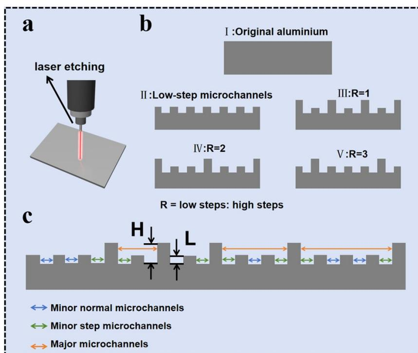
Figure. S1. (a) Schematic diagram of laser etching process. (b) Cross-section diagram of different microchannel grooves. (c) Cross-section of the layered ladder structure on the surface of different microchannels.
