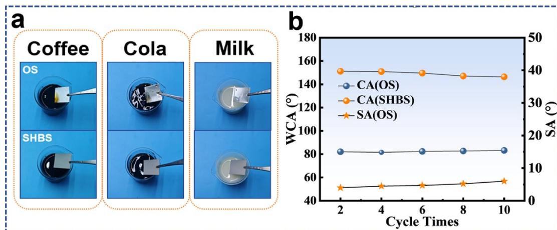
Figure. S5. (a)The antifouling properties of original substrate(OS) and superhydrophobic substrate(SHBS) in Coffee, Cola and milk, respectively.(b) (b) The effect of the anti-fouling self-cleaning performance test on the water contact angle and sliding angle of the surface of the hydrophobic substrate
