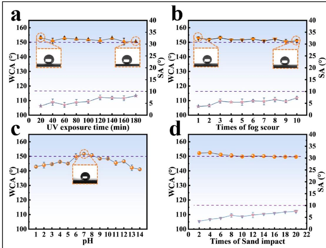
Figure. S4. (a) UV resistance test of superhydrophobic substrate (SHBS) surface. (b) Test of anti-fogging properties of superhydrophobic substrate surface. (c) Test of acid and alkali resistance on the surface of superhydrophobic substrate. (d) Sand shock test of superhydrophobic substrate surface.
