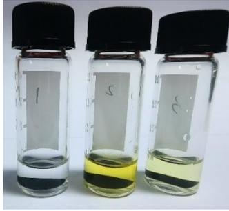
**Figure S6.** Solubility tests of *p*-PyPTZ, *p*-PzPTZ, and *p*-DzPTZ electrodes (from left to right) in the electrolyte.
