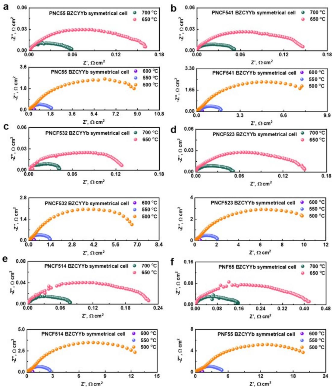
**Figure S1.** EIS of the BZCYYb-based symmetrical cells with PNC55, PNC541, PNC532, PNC523, PNC514 and PNF55 cathodes at a temperature range from 500 to 700 °C in wet air with 3 vol% H<sub>2</sub>O.
