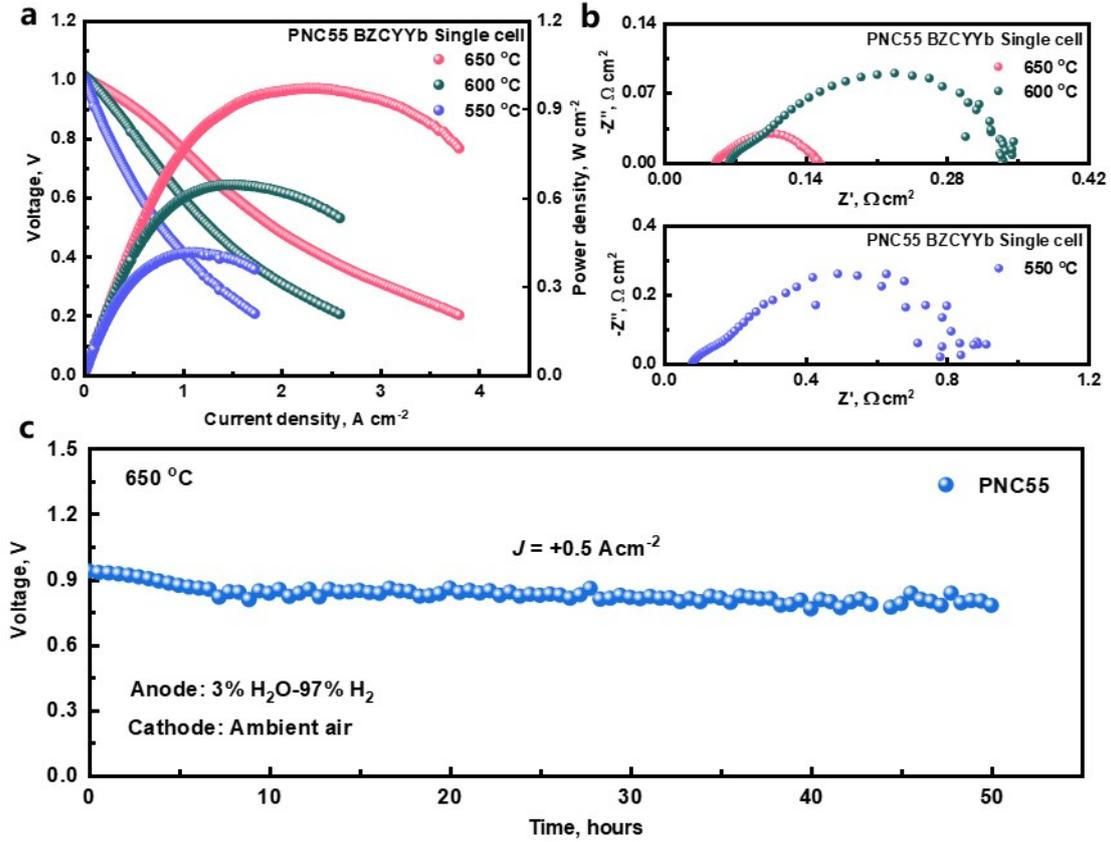
**Figure S6.** (a) Typical I-V-P curves of a single cell with PNC55 cathode measured at 650-550 °C (b) Typical EIS curves of the single cell measured at 650-550 °C under OCV conditions. (c) A short-term (~50 h) stability evaluation of the PNC55 single-cell measured at the constant current density of 0.5  $A\ cm^{-2}$  and 650 °C.
