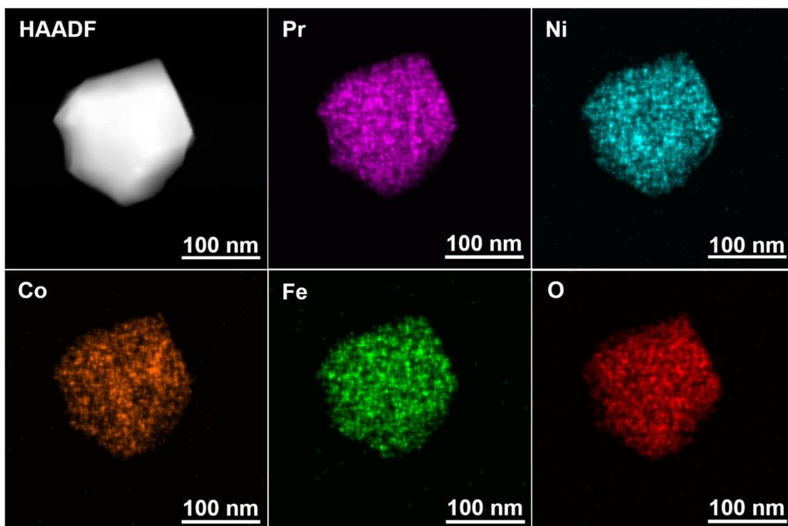
**Figure S4.** HAADF and the X-ray EDS mapping of Pr, Ni, Co, Fe and O from the PNCf532 grain.
