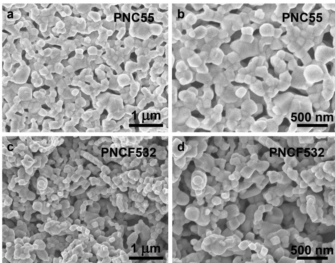
**Figure S3.** The SEM images of PNC55 and PNC532 cathodes.
