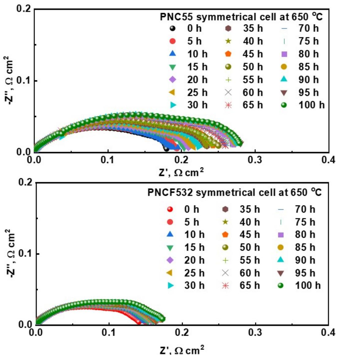
**Figure S5.** Short stability (100 h) of  $R_p$  of BZCYYb symmetrical cells with PNC55 and PNC532 cathode, tested at 650 °C under flowing air with 3 vol.%  $H_2O$ .
