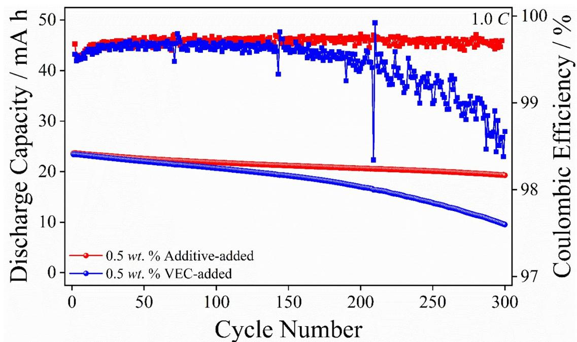
**Figure S9.** Cycleability obtained from graphite/NCM pouch cell with additive and VEC-added electrolytes
