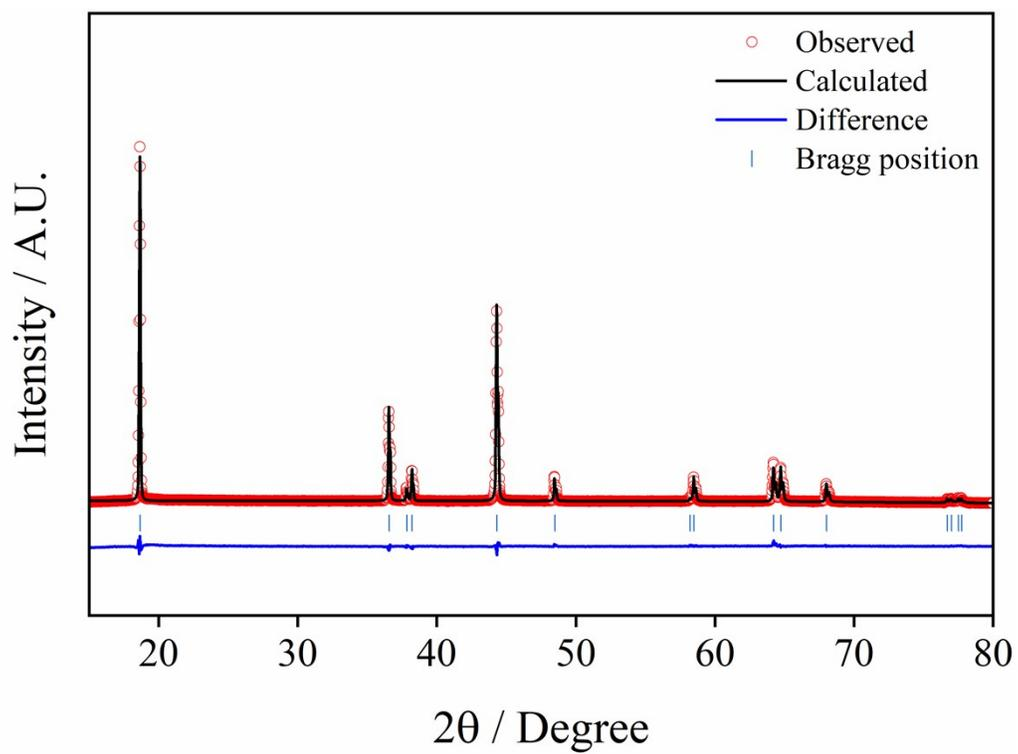
**Figure S3.** XRD spectra of synthesized NCM powder
