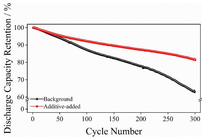
**Figure S5.** Discharge capacity retention of graphite/NCM pouch cell at 1.0 C, 2.5-4.35 V cycling condition
