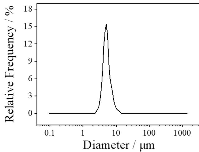
**Figure S2.** (a) SEM image and (b) particle size distribution profile of synthesized NCM powder
