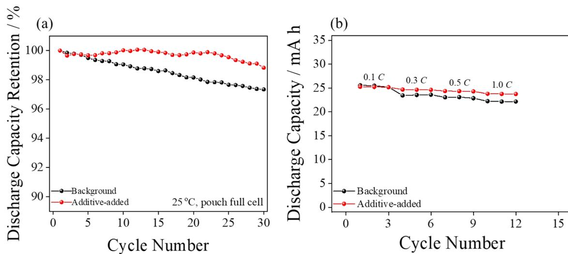
**Figure S7.** (a) cycle and (b) rate performances obtained from graphite/NCM pouch cell with background and additive-added electrolytes at 25 °C
