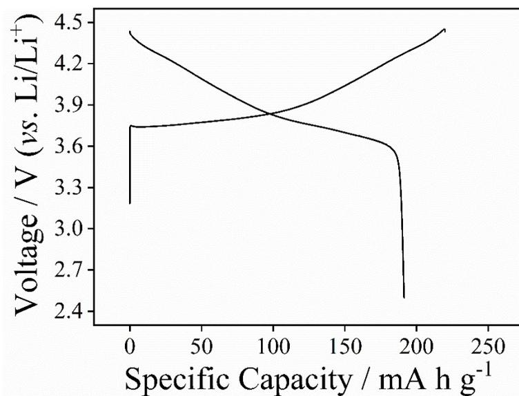
**Figure S4.** Li half-cell initial voltage profile of synthesized NCM electrode at areal capacity of 2.5 mA h cm<sup>-2</sup>
