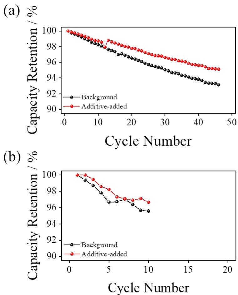
**Figure S8.** Coin half-cell cycle performances of (a) NCM and (b) graphite electrodes with background and additive-added electrolytes at 25 °C and 0.5 *C*-rate
