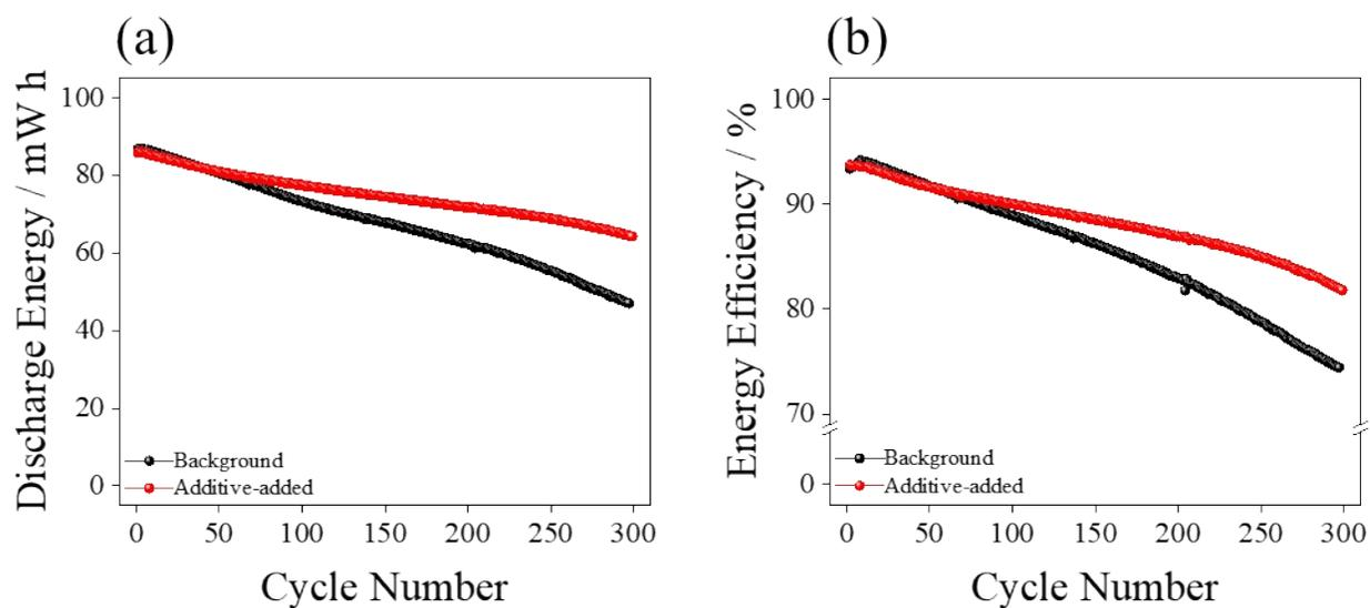
**Figure S6.** (a) Discharge energy and (b) energy efficiency of graphite/NCM cells with background and additive-added electrolytes, respectively
