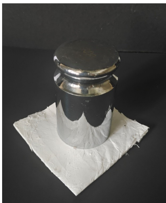
Fig. S7. Photograph of a 500 g weight placed on the LCGESZ-SiO 2 membrane
