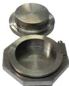
Figure S1: A heat compression mold with a diameter of 5 cm was used for the reprocessing of the vitrimers.
