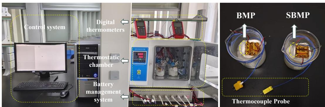
18 Figure S4. Optical images of high temperature thermal management experiment set-up
