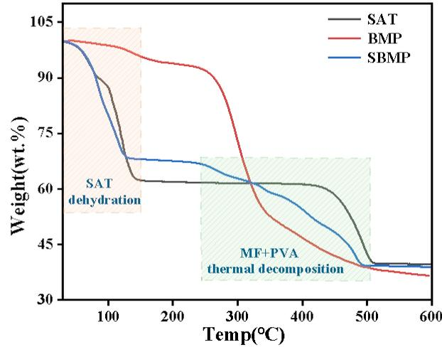
21 Figure S7. TGA curves of SAT, BMP and SBMP
