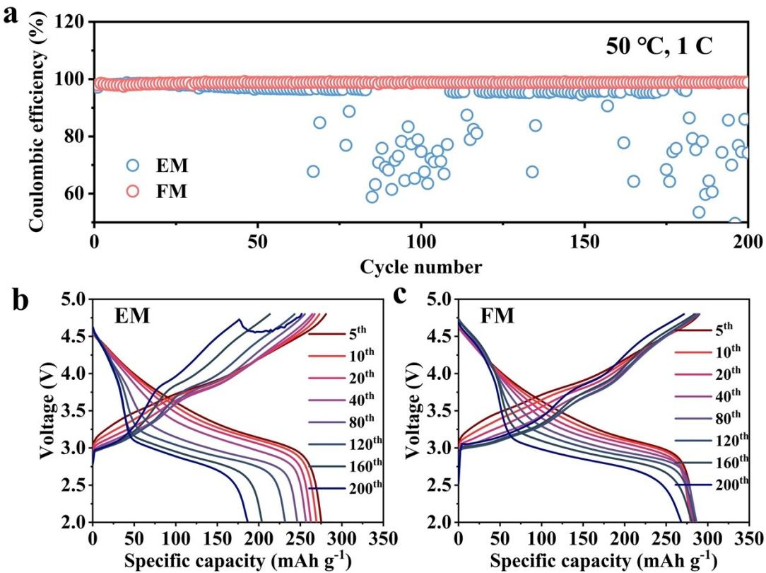
**Fig. S8.** (a) Coulombic efficiency of Li||LRM cells using different electrolytes at 50 °C. (b, c) Corresponding charge and discharge curves with (b) EM and (c) FM electrolytes.
