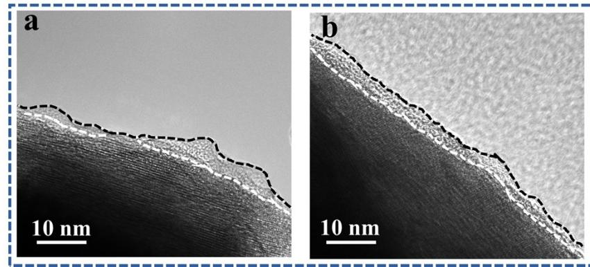
**Fig. S10.** TEM images of LRM cathode materials with (a) EM and (b) FM electrolytes after 100 cycles.
