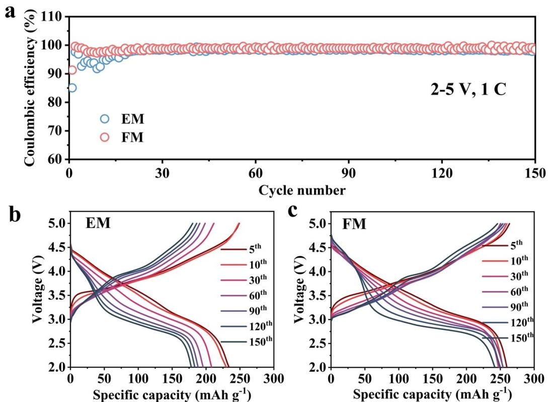
**Fig. S7.** (a) Coulombic efficiency of Li||LRM cells using different electrolytes in the voltage range of 2-5 V. (b, c) Corresponding charge and discharge curves with (b) EM and (c) FM electrolytes.
