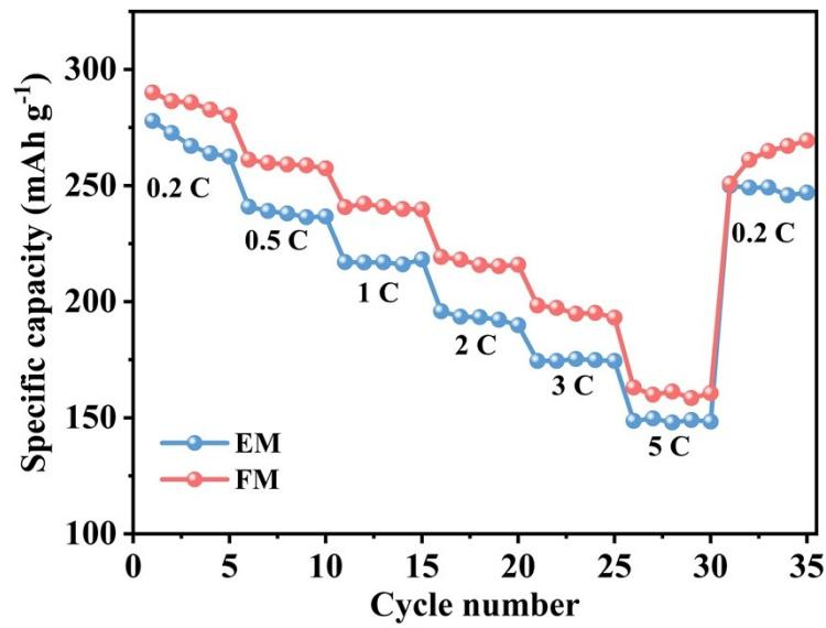
**Fig. S5.** Rate capability of Li||LRM cells with different electrolytes at 0.2, 0.5, 1, 2, 3, 5, and 0.2 C.
