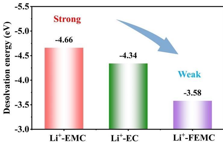
**Fig. S3.** The desolvation energies based on the coordination numbers between  $\text{Li}^+$  and solvents.
