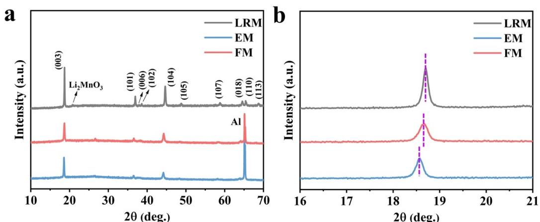
**Fig. S9.** The XRD patterns of the pristine LRM cathode and the cycled cathodes with EM and FM electrolytes. (b) Corresponding enlarged local plots.
