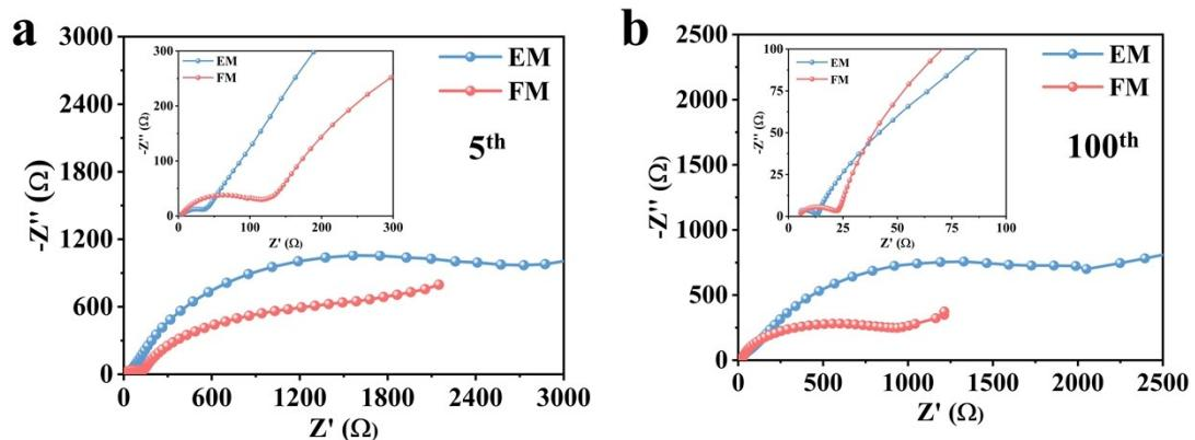
**Fig. S6.** Nyquist plots of Li||LRM cells using EM and FM electrolytes after 5 and 100 cycles, respectively.
