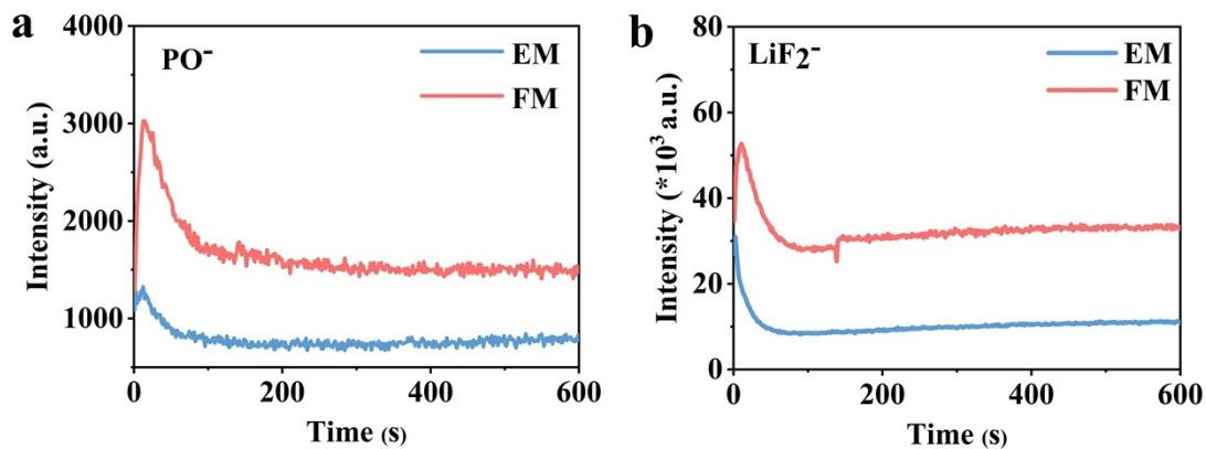
**Fig. S12.** The etching depth curves of the cycled cathode with different electrolytes by  $\text{PO}^-$  and  $\text{LiF}_2^-$ .
