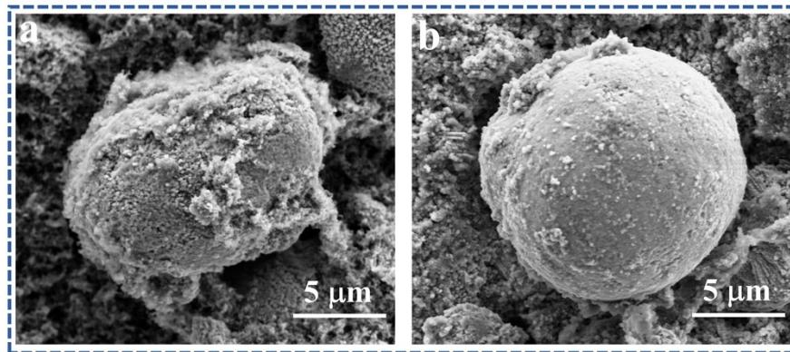
**Fig. S11.** SEM images of LRM cathode materials with (a) EM and (b) FM electrolytes after 100 cycles.
