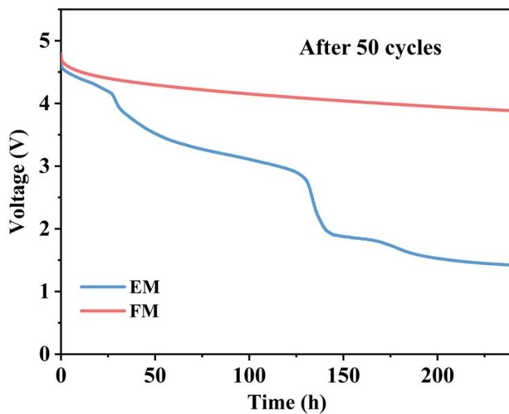
**Fig. S4.** Self-discharge curves of  $\text{Li} \parallel \text{LRM}$  cells with EM and FM electrolytes at 4.8 V after 50 cycles.
