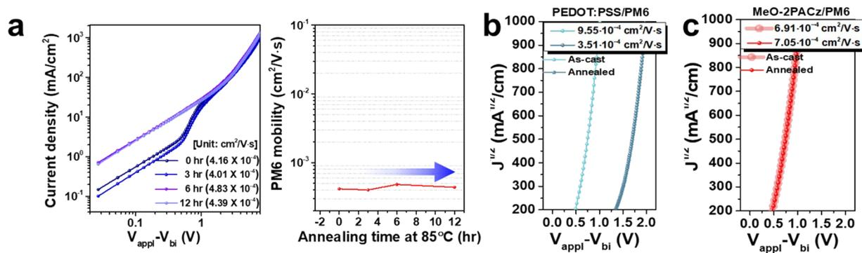
**Figure S9.** SCLC plots of (a) 0.5 mg/ml PM6 over aging time at 65 °C. SCLC plots of (b) as-cast and annealed PEDOT:PSS/PM6 and (c) as-cast and annealed MeO-2PACz/PM6 at 65 °C for 12 hours.
