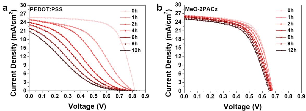
**Figure S10.** Time-dependent J–V curves of a representative device from the stability tests of ITO/HTL/PM6:Y6/PFN-Br/Ag structures using (a) PEDOT:PSS and (b) MeO-2PACz as the HTL.
