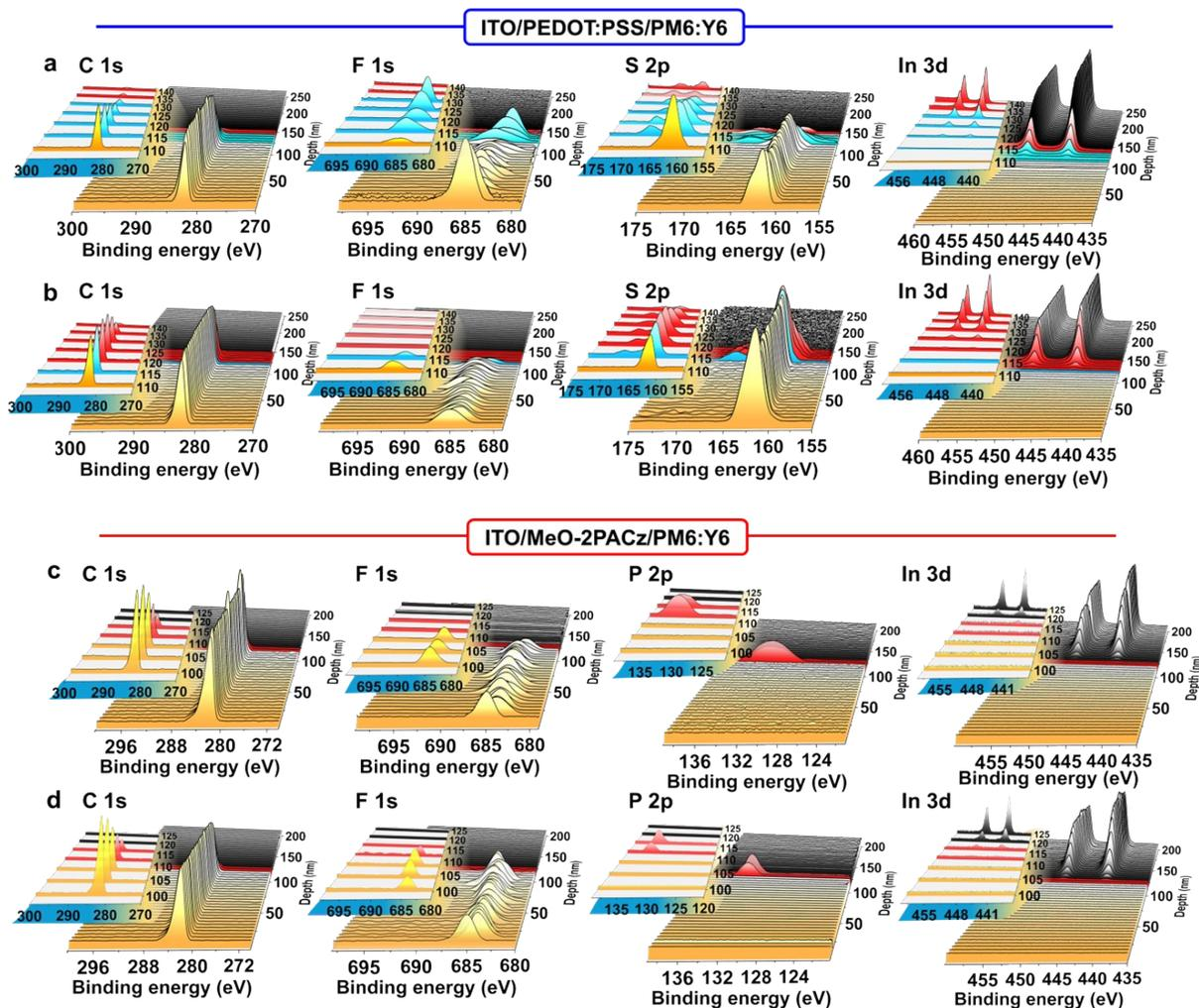
**Figure S7.** Depth profile XPS spectra of (a) pristine ITO/PEDOT:PSS/PM6:Y6 film, (b) annealed ITO/PEDOT:PSS/PM6:Y6 film at 65 °C for 12 hours, (c) pristine ITO/MeO-2PACz/PM6:Y6 film and (d) annealed ITO/MeO-2PACz/PM6:Y6 film at 65 °C for 12 hours.
