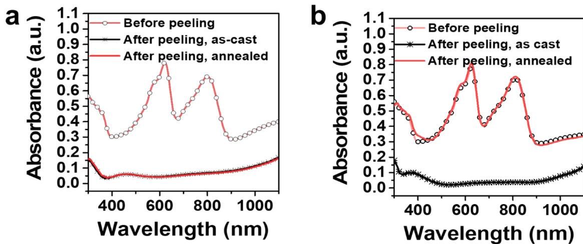
**Figure S4.** UV-vis absorption spectra before and after the peeling test of (a) PEDOT:PSS/PM6:Y6 and (b) MeO-2PACz/PM6:Y6 films.
