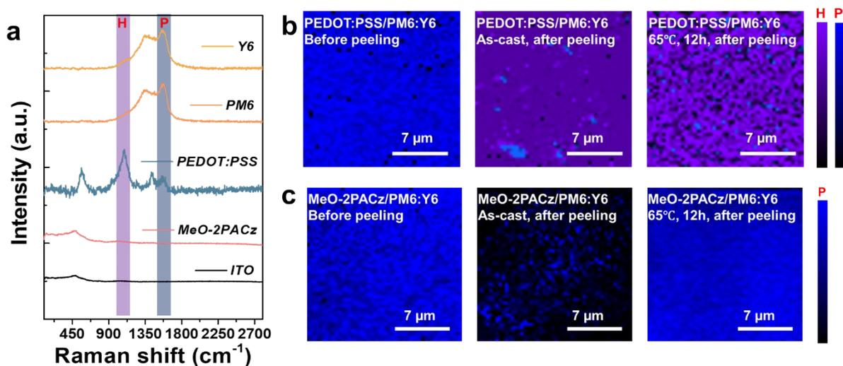
**Figure S5.** (a) Pristine Raman results of Y6, PM6, PEDOT:PSS, the SAM, and ITO substrate. Here, H and P represent the peak points of PEDOT:PSS and PM6:Y6, respectively, and are indicated in purple and blue in the Raman image. The films of (b) PEDOT:PSS/PM6:Y6 and (c) MeO-2PACz/PM6:Y6 before and after the peeling test.
