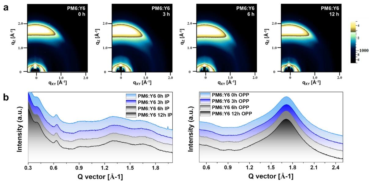
**Figure S3.** (a) GIWAXS diffraction patterns and (b) GIWAXS linecut profiles of PM6:Y6 film over time at 65°C. The abbreviations IP and OPP denote *in-plane* and *out-of-plane*, respectively.
