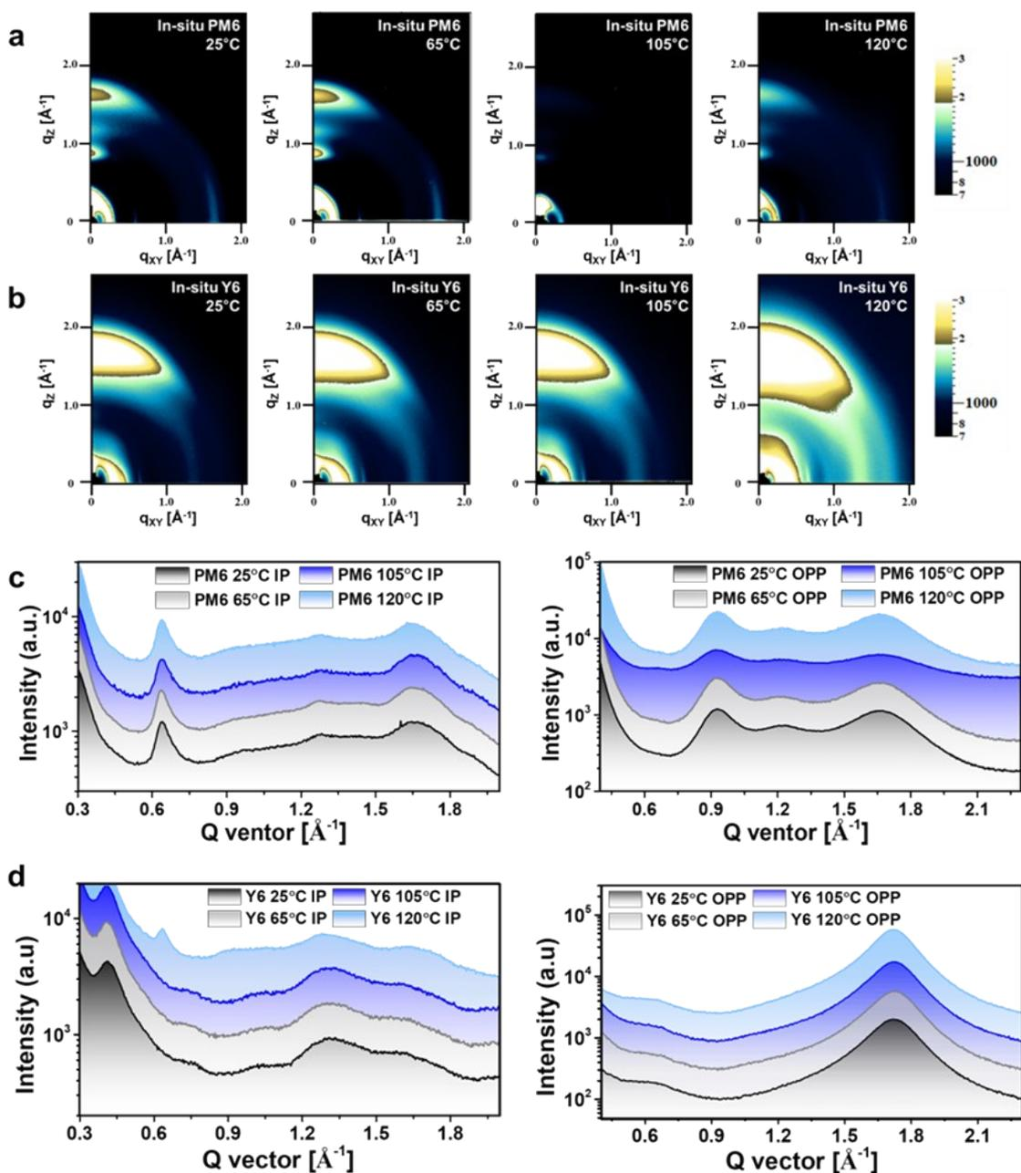
**Figure S2.** *In-situ* GIWAXS of (a) PM6 and (b) Y6. The (c) *in-plane* and (d) *out-of-plane* line-cut profiles of PM6 and Y6 extracted from the 2D GIWAXS patterns. The abbreviations IP and OPP denote *in-plane* and *out-of-plane*, respectively.
