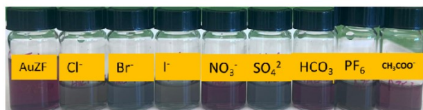
Figure S6. (a) Absorbance measurements of the AuZnFe 2 O 4 nanocomposite in the presence of different interferences and (b) the corresponding color changes. Interferents were tested at 0.30 M (Cl - , Br - , I - , NO 3 - , SO 4 2- , HCO 3 - , F 6 - , and CH 3 COO - ).
