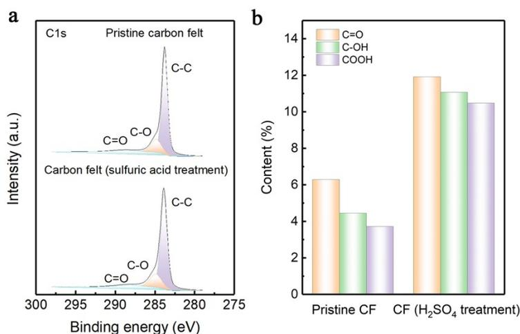
Figure S20 (a) The high-resolution C 1s XPS spectra of the pristine carbon felt and carbon felt treated in sulfuric acid. (b) Elemental composition and content of oxygen functional groups on the samples.
