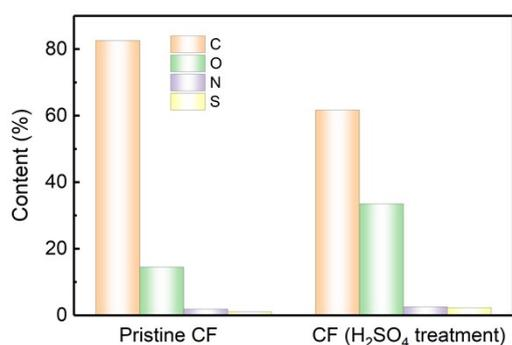
Figure S19 Composition and content of elemental on the pristine carbon felt and carbon felt treated in sulfuric acid.
