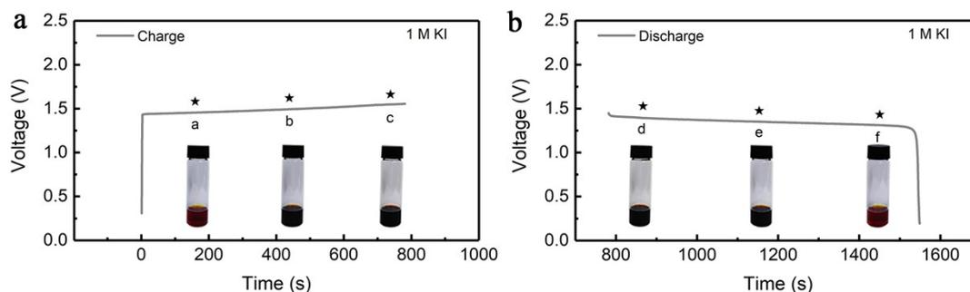
Figure S10 (a) charge and (b) discharge curves and their corresponding photographs of the KI electrolyte at different stages.
