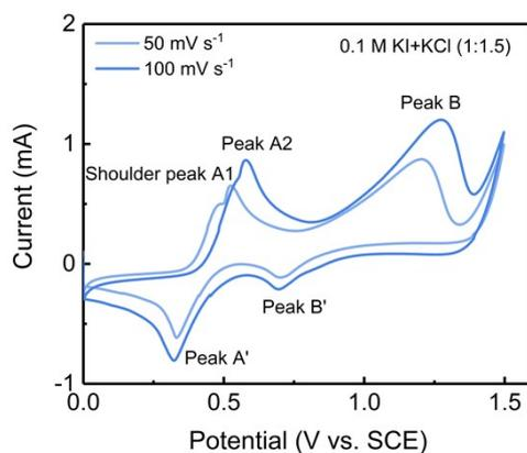
Figure S3 Cyclic voltammograms of redox reactions in 0.1 M KI+KCl (1:1.5) electrolyte at different scan rates.
