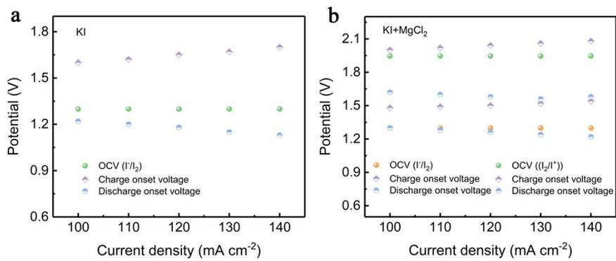
Figure S27 The charge and discharge onset voltage of (a) KI and (b) KI+MgCl<sub>2</sub> electrolytes at different current density.
