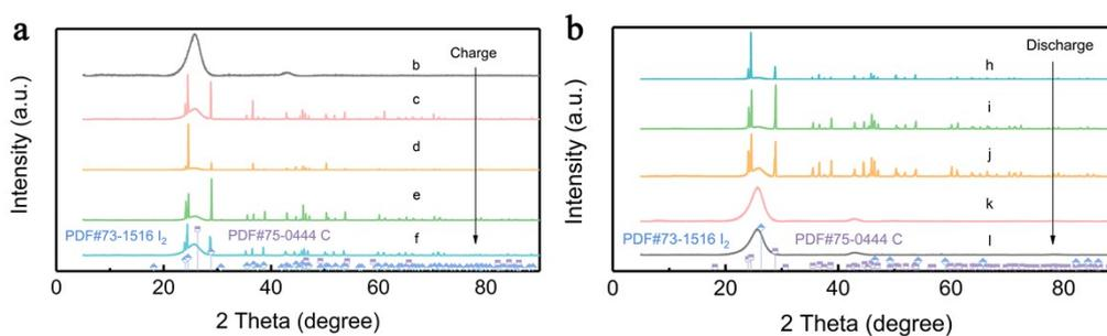
Figure S18 XRD spectra of the products from (a) charge and (b) discharge steps in KI+KCl (1:1) electrolytes.
