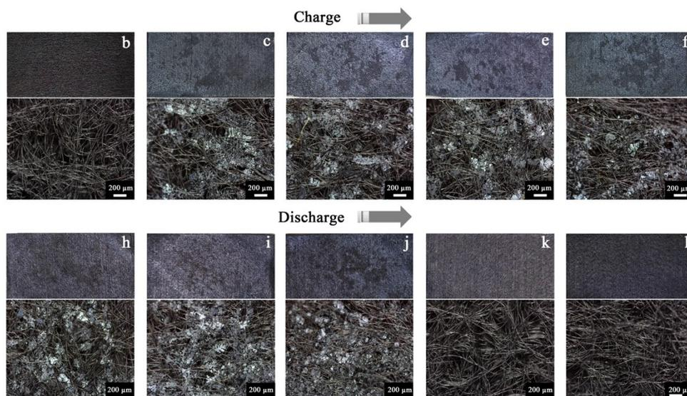
Figure S17 The morphologies of iodine species on carbon felt in KI+KCl (1:1) electrolyte at charge and discharge stages in a battery system.
