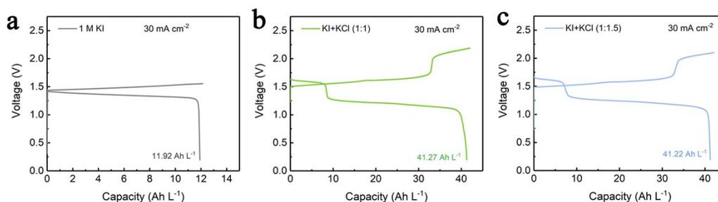
Figure S7 Galvanostatic voltage profiles of the ZIFB with (a) KI, (b) KI+KCl (1:1) and (c) KI+KCl (1:1.5) electrolytes as polysolite at a current density of 30 mA cm<sup>-2</sup>.
