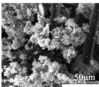
Figure S24 Cross-sectional SEM images of the carbon felt after long cycling.
