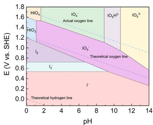
Figure S6 E-pH diagram of I-H<sub>2</sub>O system.
