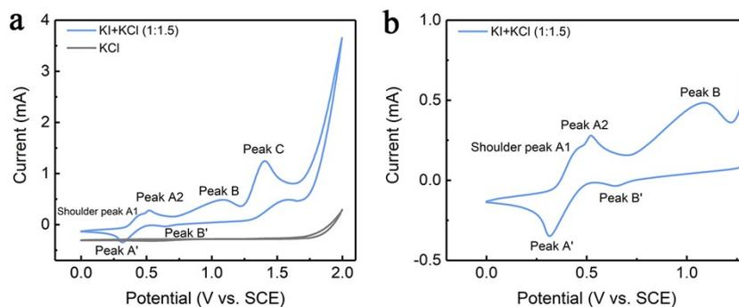
Figure S2 (a) Cyclic voltammograms of redox reactions in pristine KI+KCl (1:1.5) and KCl electrolytes at a scan rate of  $20 \text{ mV s}^{-1}$ ; (b) Magnification of (a).
