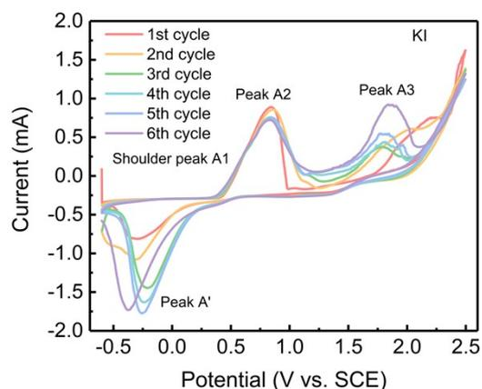
Figure S1 Cyclic voltammograms of redox reactions in pristine KI electrolyte at a scan rate of 20 mV s<sup>-1</sup>.
