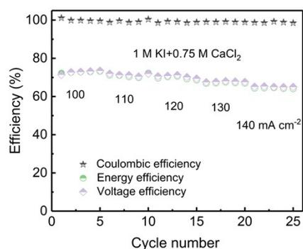
Figure S25 Rate performance of the ZIFB adopting 1 M KI+0.75 M CaCl<sub>2</sub> electrolytes cycled at various current densities from 100 mA cm<sup>-2</sup> to 140 mA cm<sup>-2</sup>.
