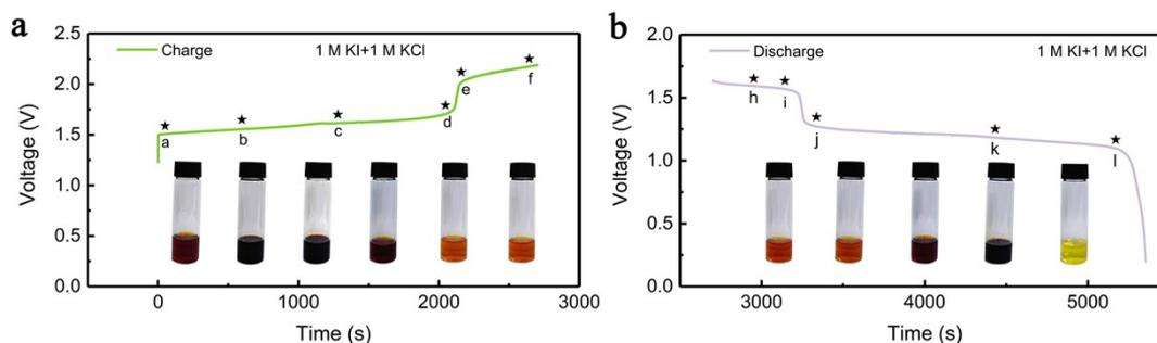
Figure S11 (a) charge and (b) discharge curves and their corresponding photographs of the KI+KCl (1:1) electrolyte at different stages.
