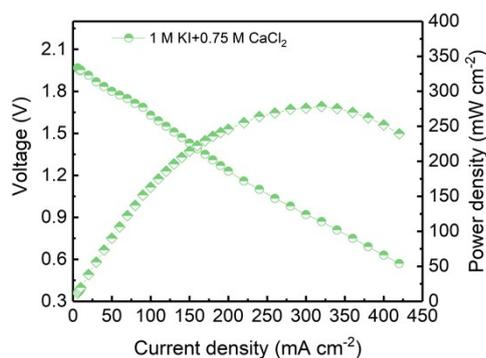
Figure S26 Discharge polarization and calculated power density curves of the ZIFB with 1 M KI+0.75 M CaCl<sub>2</sub> electrolytes at a state of charge (SOC) of 90%.
