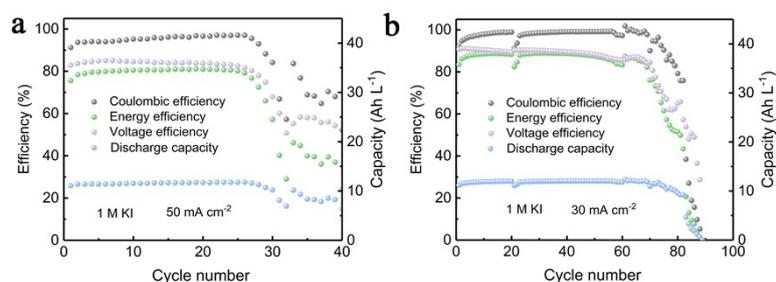
Figure S9 The discharge capacity and efficiencies of ZIFB using KI electrolytes at a current density of (a)  $50 \text{ mA cm}^{-2}$  and (b)  $30 \text{ mA cm}^{-2}$ .
