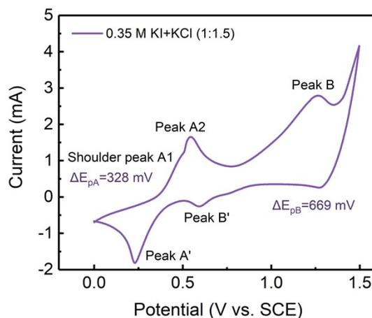
Figure S4 Cyclic voltammograms of redox reactions in 0.35 M KI+KCl (1:1.5) electrolyte at a scan rate of  $100 \text{ mV s}^{-1}$ .
