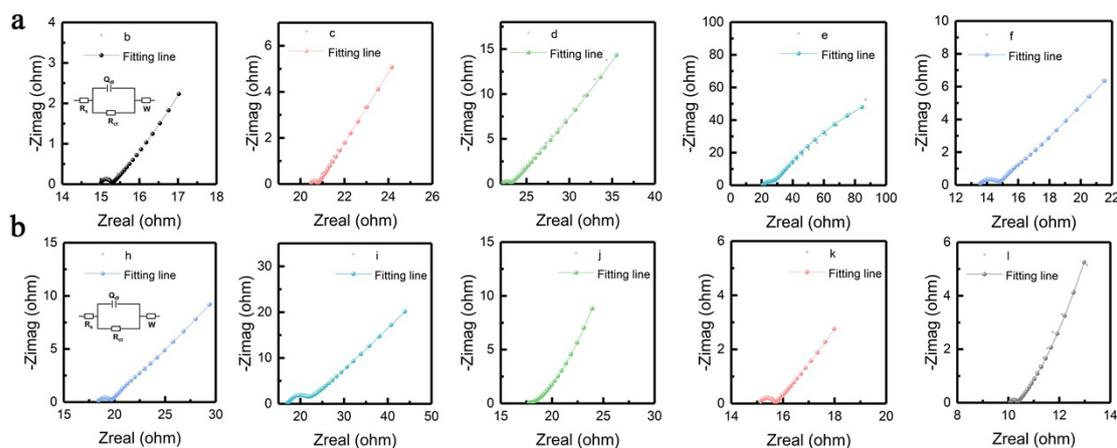
Figure S22 EIS results of the ZIFB at (a) charge and (b) discharge stages in KI+KCl (1:1) electrolytes.
