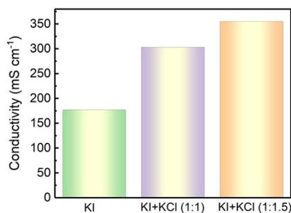
Figure S8 Conductivity of three aqueous electrolytes with different concentrations of Cl<sup>-</sup> additives.
