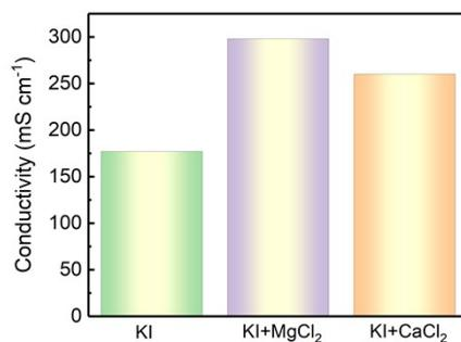
Figure S23 Conductivity of various electrolytes.
