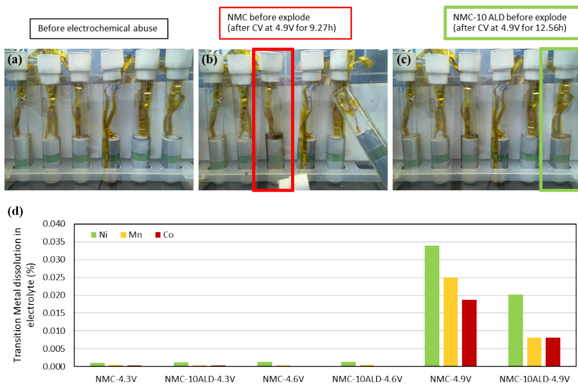
Fig. S15 The jelly roll showing color of electrolyte at (a) before abuse, (b) before explosion of NMC after abused at 4.9V, and (c) before explosion of NMC-10ALD after abused at 4.9V. (d) Transition metal dissolution in electrolyte
