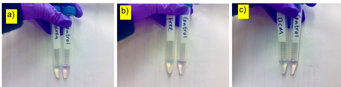
Figure S10. Permanganate test for \text{H}_2\text{O}_2 product produced from TiN synthesized from: a) the urea-glass method TiN, b) a direct solventless reaction, and c) a \text{TiCl}_4(\text{OC}(\text{NH}_2)_2)_2 complex.
