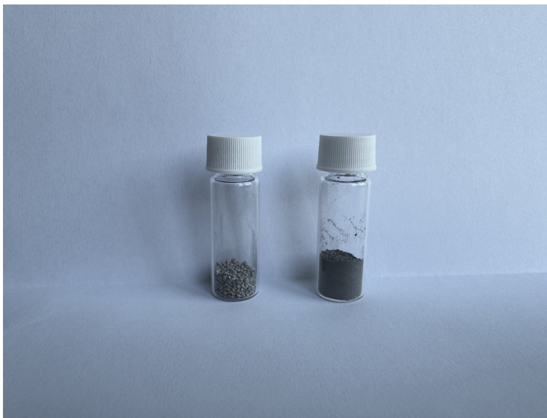
Fig. S2 Photos of as-received (left) and activated (right) 3 g TiCrMnFeZr HEA sample.
