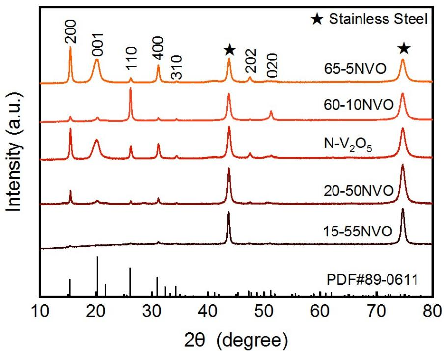
Fig. S3 XRD patterns of the 15-55NVO, 20-50NVO,  $\text{N-V}_2\text{O}_5$ , 60-10NVO, and 65-5NVO thin films.
