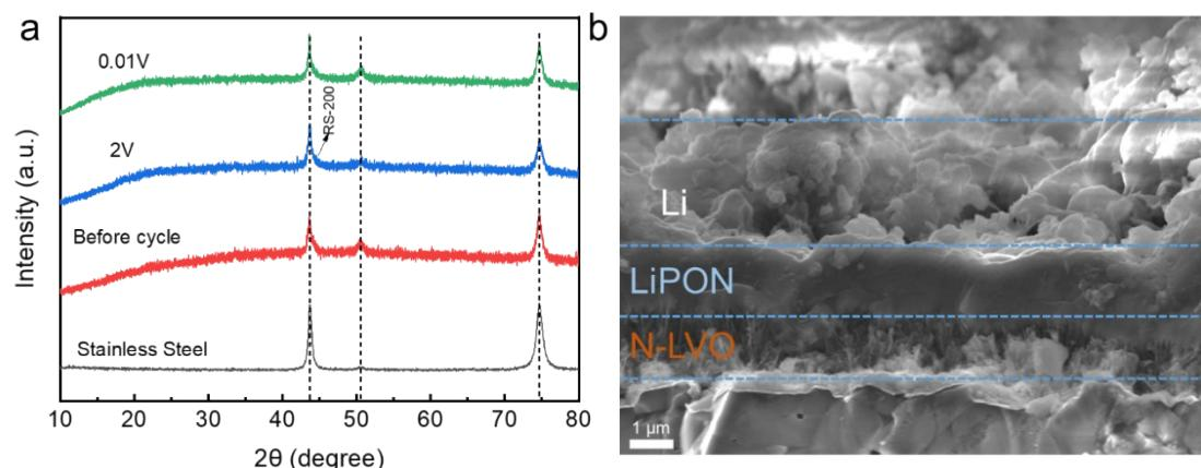
Fig. S13. (a) XRD patterns of the N-LVO TFB before cycle and at 2 V and 0.01 V states after 200 cycle. (b) Cross-sectional FESEM image of the N-LVO TFB after 200 cycles. (For the XRD measurement, the Li anode in the N-LVO TFB was pre-removed by using ethanol.)
