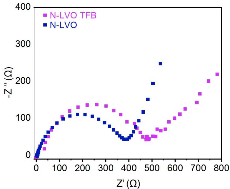
Fig. S12. Comparison of the EIS spectra of the N-LVO TFB and the N-LVO electrode.
