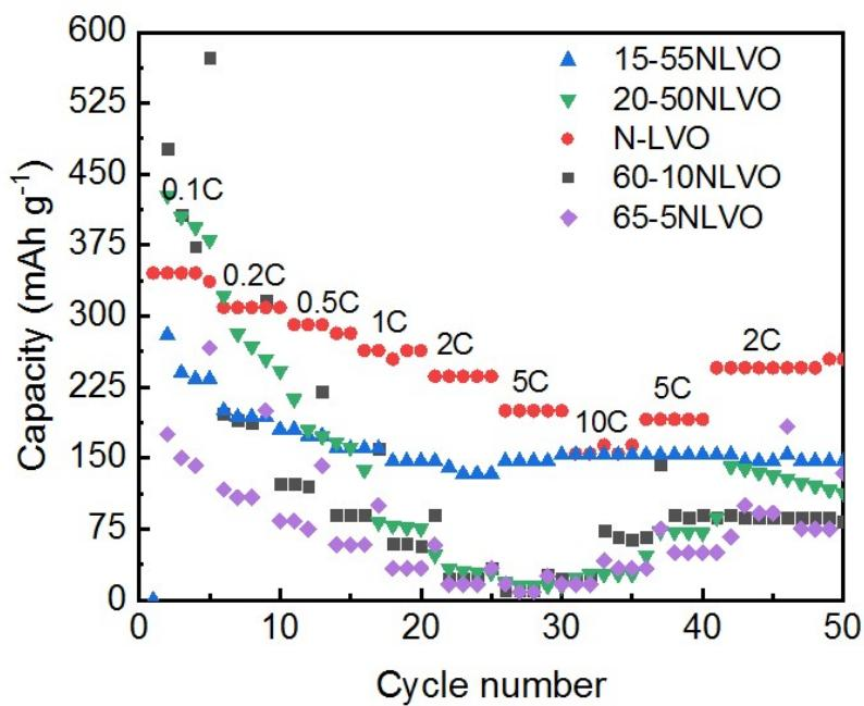
Fig. S8 Rate performances of the 15-55NLVO, 20-50NLVO, N-NLVO, 60-10NLVO, and 65-5NLVO electrodes.
