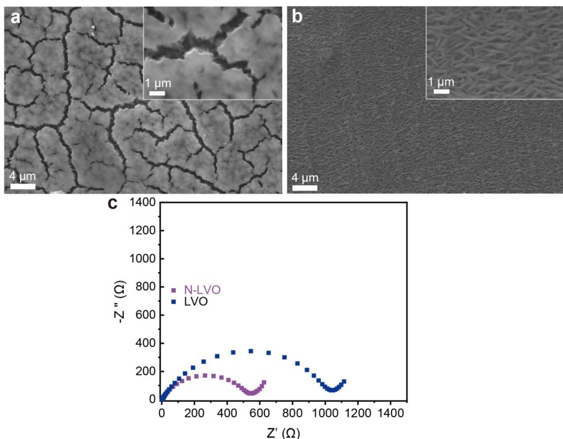
Fig. S9 Top-view FESEM images of the (a) LVO and (b) N-LVO electrodes after 50 cycles. (c) EIS spectra of the LVO and N-LVO electrodes after 50 cycles.
