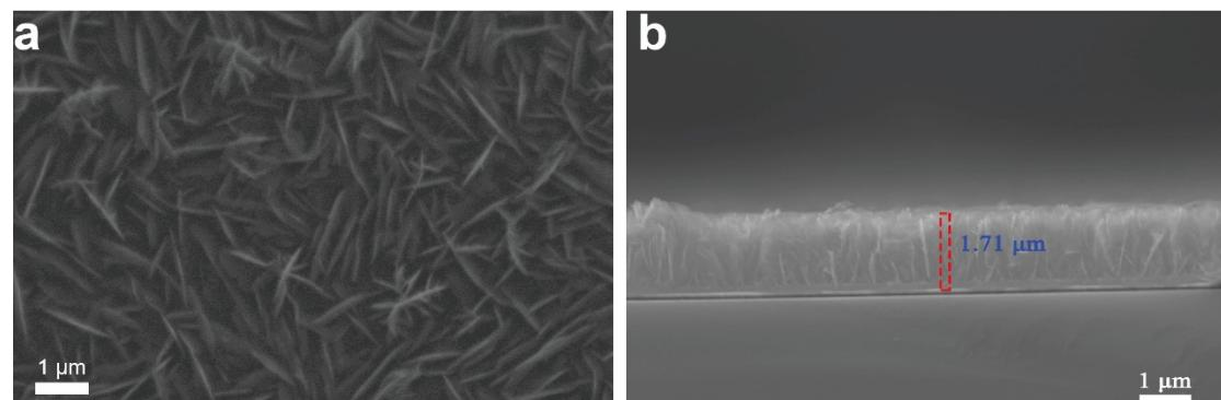
Fig. S1 (a) Top-view FESEM image and (b) cross-sectional FESEM image of the  $\text{V}_2\text{O}_5$  thin film.
