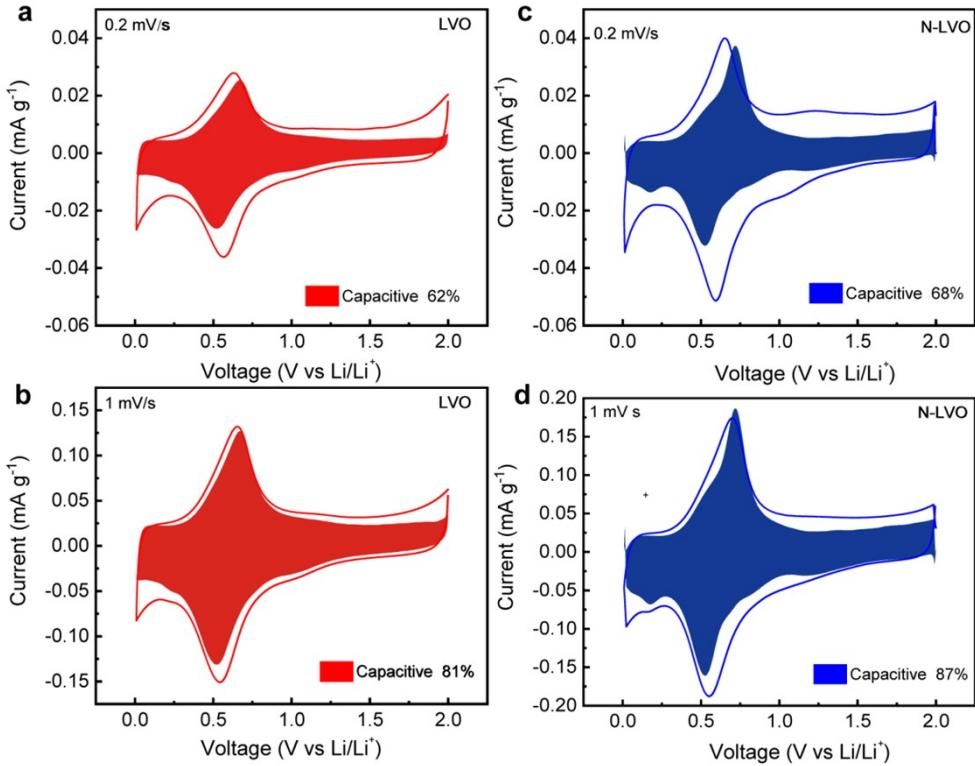
Fig. S10 CV curves of the LVO electrode at scan rates of (a)  $0.2 \text{ mV s}^{-1}$  and (b)  $1 \text{ mV s}^{-1}$  with shade region representing capacitive capacity contribution. CV curves of the N-LVO electrode at scan rates of (c)  $0.2 \text{ mV s}^{-1}$  and (d)  $1 \text{ mV s}^{-1}$  with shade region representing capacitive capacity contribution.
