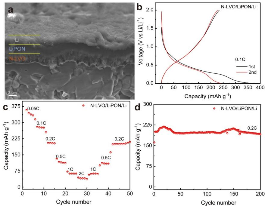
Fig. S11 (a) Cross-sectional FESEM image, (b) initial two charge and discharge curves at  $0.1\text{C}$ , (c) rate performance, and (d) cycle performance at  $0.2\text{C}$  of the N-LVO TFB.
