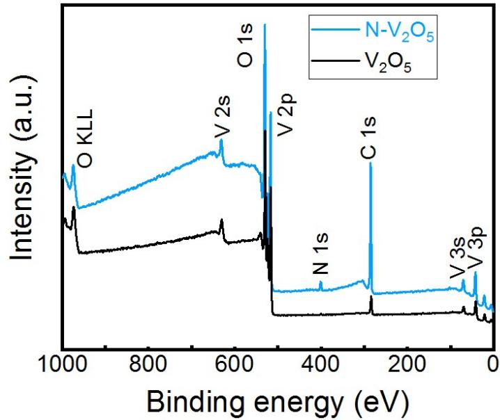
Fig. S6 Survey scan XPS spectra of the  $\text{N-V}_2\text{O}_5$  and  $\text{V}_2\text{O}_5$  thin films.
