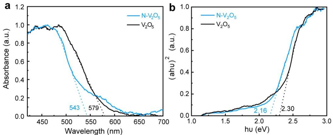
Fig. S7 (a) UV–vis absorption spectra and (b) the transformed Kubelka–Munk function against the photon energy plots of the  $\text{N-V}_2\text{O}_5$  and  $\text{V}_2\text{O}_5$  thin films.
