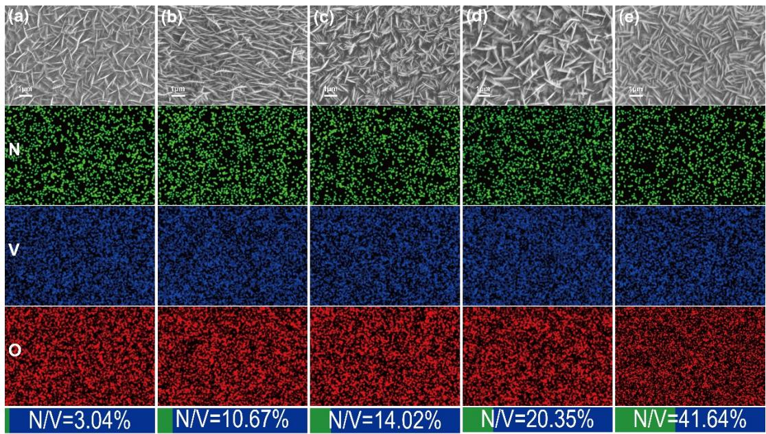
Fig. S4 FESEM images and EDS elemental mapping images of the (a) 15-55NVO, (b) 20-50NVO, (c) N-V<sub>2</sub>O<sub>5</sub>, (d) 60-10NVO, and (e) 65-5NVO thin films.
