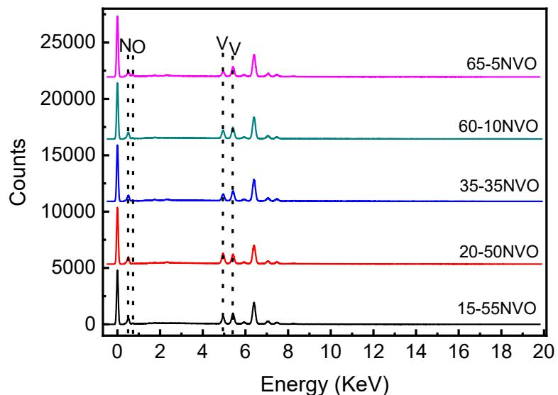
Fig. S5 EDS spectra of the 15-55NVO, 20-50NVO, N-V<sub>2</sub>O<sub>5</sub>, 60-10NVO, and 65-5NVO thin films.
