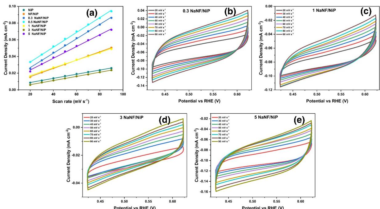
**Figure S4.** (a) Scan rate vs. Current density plot of NaNF/NiP electrodes, (b-e) CV in the non-faradaic region of NaNF/NiP electrodes
