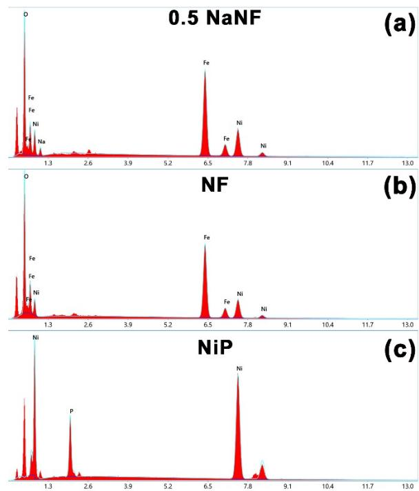
**Figure S1.** EDAX spectra of (a) 0.5 NaNF powder, (b) NF powder, and (c) NiP electrode
