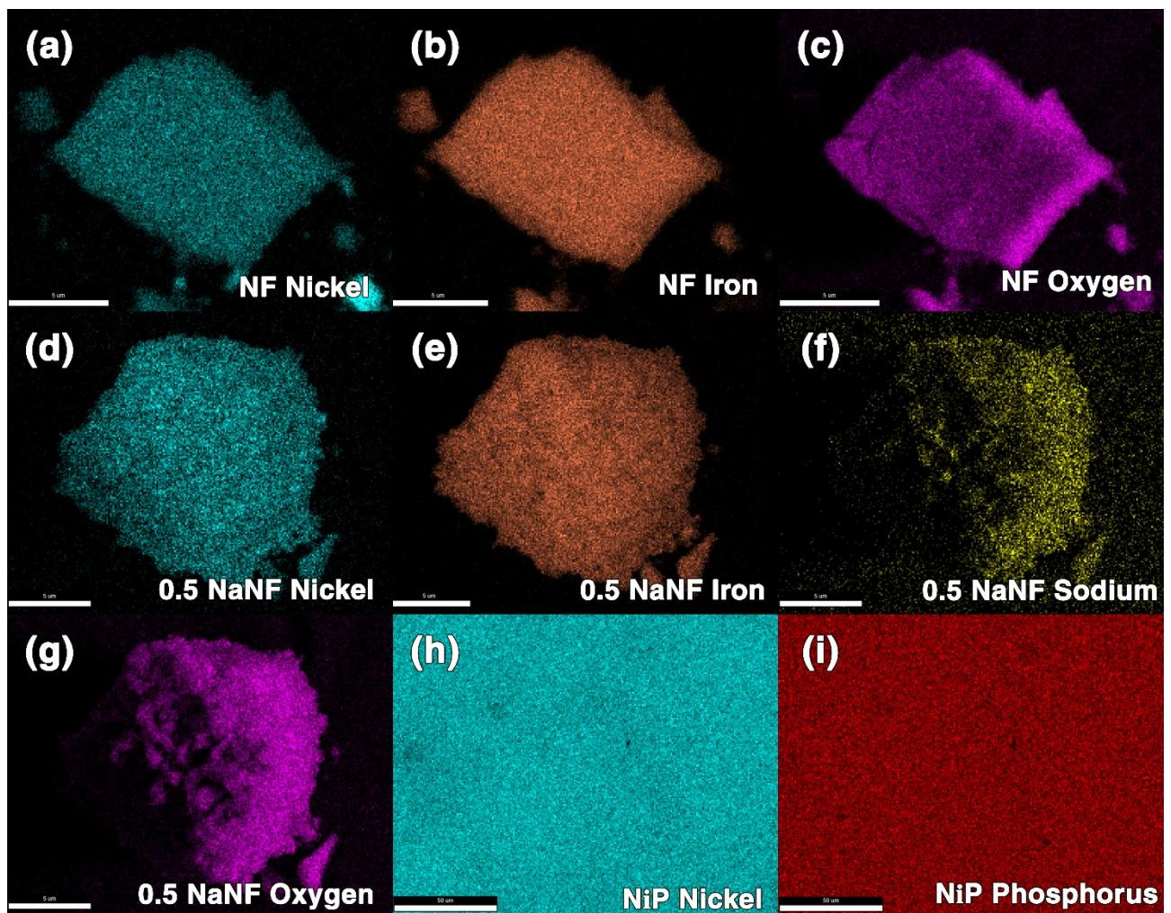
**Figure S2.** Elemental mapping NF powder, 0.5 NaNF powder and NiP electrode
