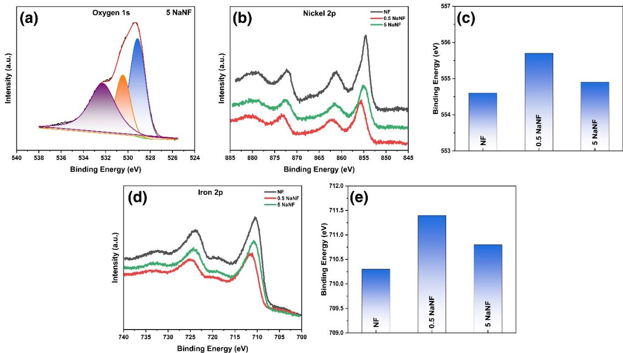
**Figure S3.** (a) Deconvoluted O 1s XPS spectra of 5 NaNF, (b) Ni 2p XPS spectra, (c) Binding energies of Ni2p (d) Fe 2p XPS spectra, (e) Binding energies of Fe2p XPS spectra
