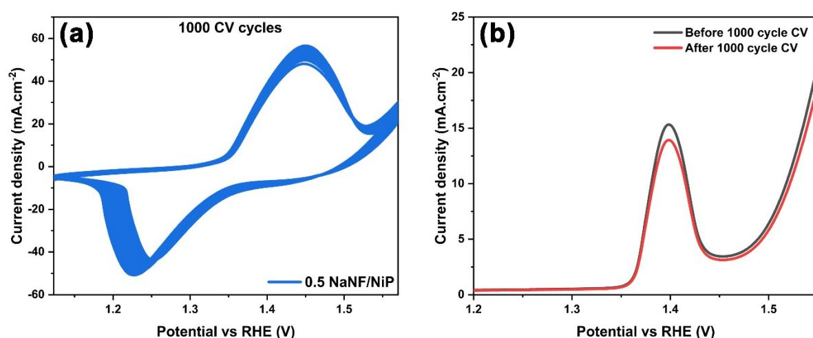
**Figure S6.** (a) 1000 CV cycles in the NiOOH redox potential, (b) LSV before and after the 1000 cycle CV study
