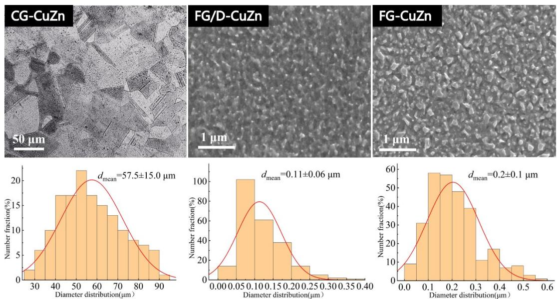
**Fig. S1** OM/SEM images of CG-CuZn, FG/D-CuZn and FG-CuZn, and the corresponding statistical chart of average grain sizes.
