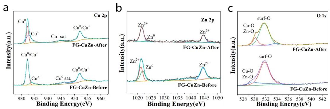
**Fig. S9** XPS spectra of FG-CuZn before and after 30 min of CO<sub>2</sub>RR: (a) Cu 2p; (b) Zn 2p; (c) O 1s.
