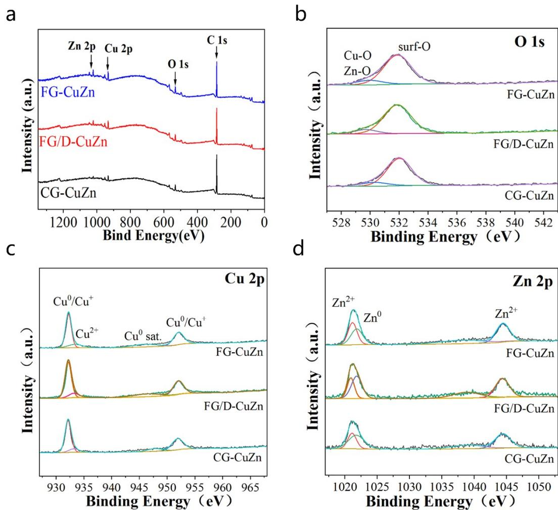
**Fig. S8** XPS of CG-CuZn, FG/D-CuZn and FG-CuZn: (a) survey spectrum; (b) O 1s; (c) Cu 2p; (d) Zn 2p.
