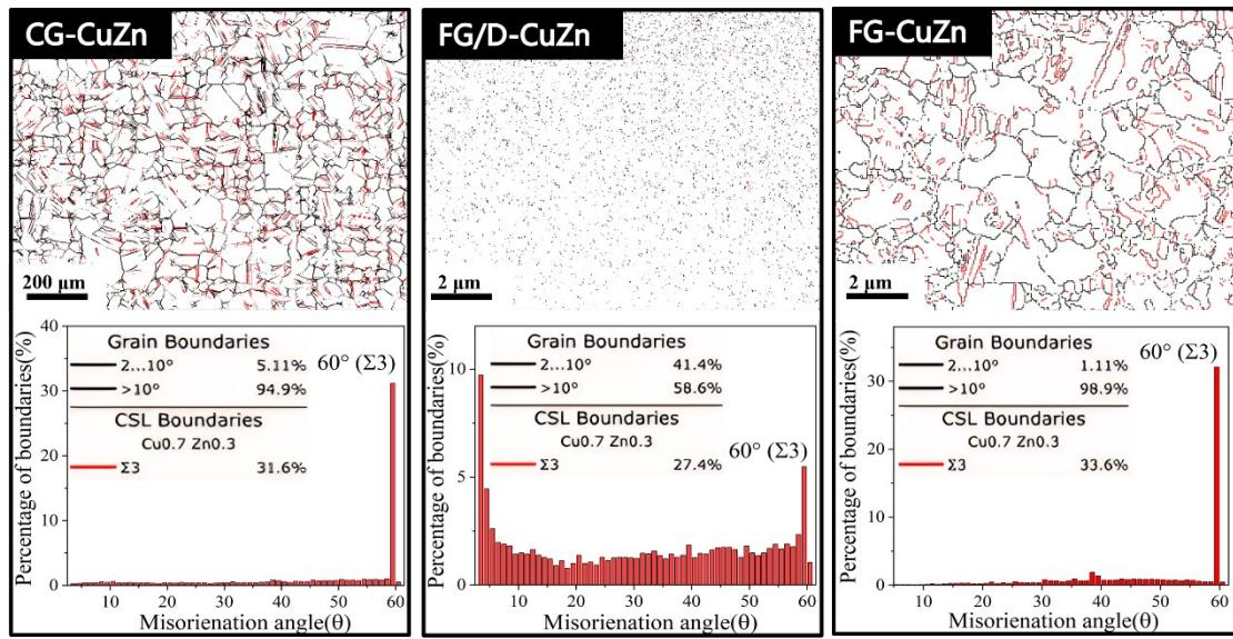
**Fig. S3** grain boundary diagrams and misorientation angle distribution diagrams of EBSD for CG-CuZn, FG/D-CuZn and FG-CuZn samples. The black lines represent general grain boundaries, and the red lines represent twin grain boundaries ( $\Sigma 3$ ).
