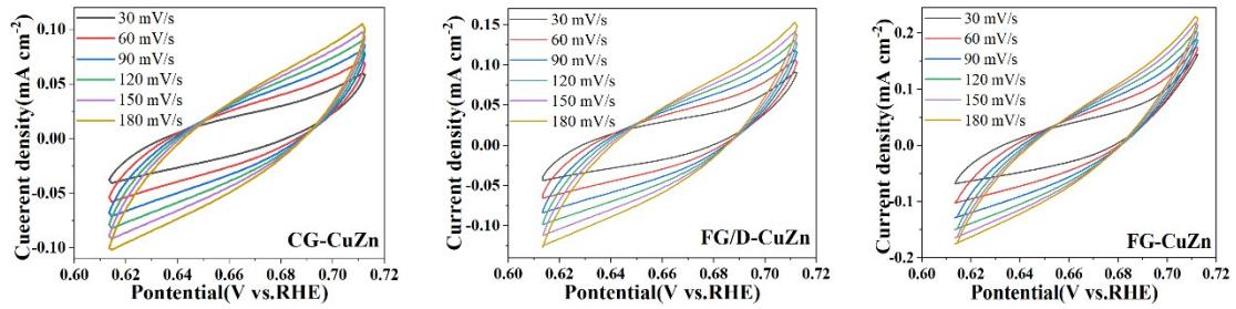
**Fig. S5** The CV of CG-CuZn, FG/D-CuZn and FG-CuZn at different scan rates.
