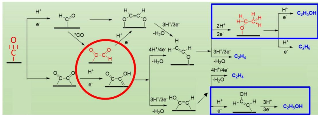
**Fig. S7** The generation pathway diagram of  $\text{C}_2+$  products ( $\text{C}_2\text{H}_4$ ,  $\text{C}_2\text{H}_5\text{OH}$ ,  $\text{C}_2\text{H}_6$ ) in the electrocatalytic  $\text{CO}_2\text{RR}$ .
