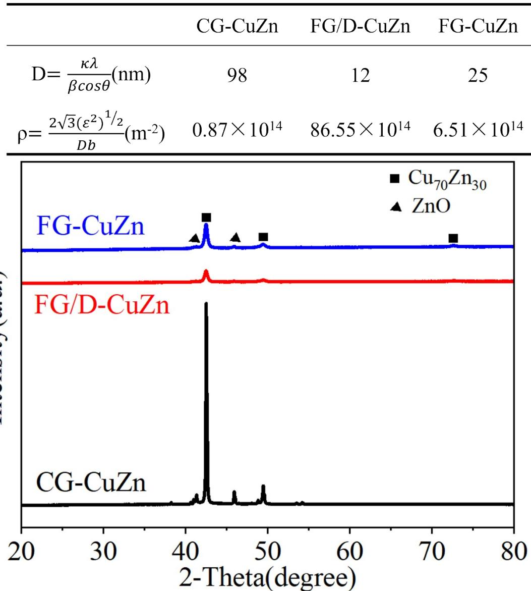
**Fig. S2** XRD patterns of CG-CuZn, FG/D-CuZn and FG-CuZn, and the corresponding calculation results of crystallite size ( $D$ ) and dislocation density ( $\rho$ )
