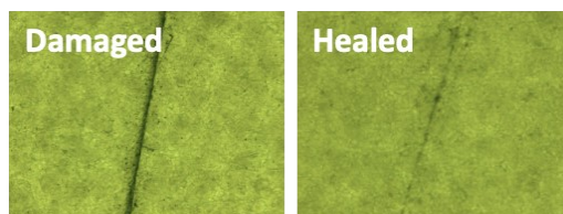
Figure S11 Healing process of the BMSHPU-30 was observed by the optical microscope.
