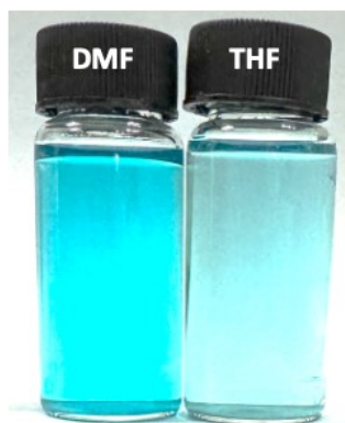
Figure S15 Optical images of BMSHPU-30 after immersion in DMF and THF solvents.
