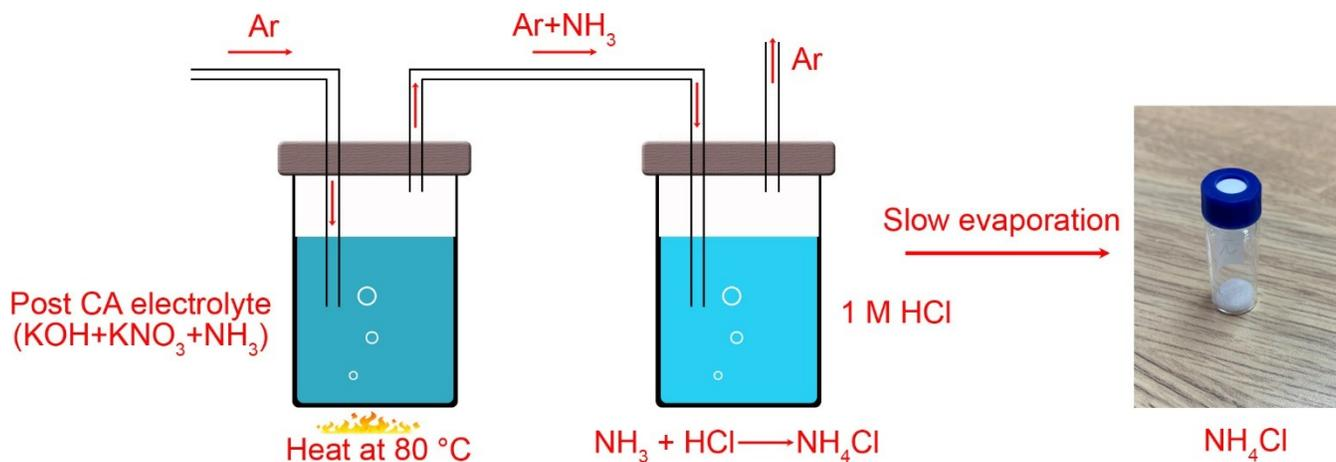
**Figure S25.** Systematic illustrating the acid stripping process to trap NH<sub>3</sub> and generate NH<sub>4</sub>Cl powder.
