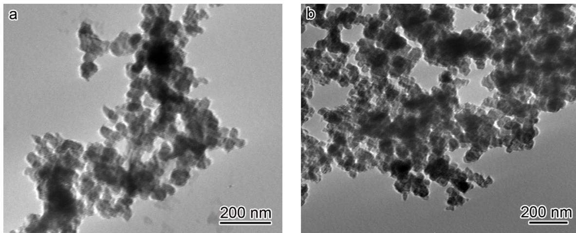
**Figure S1.** (a) TEM image of CuBr-N/CB and (b) CuI-N/CB.
