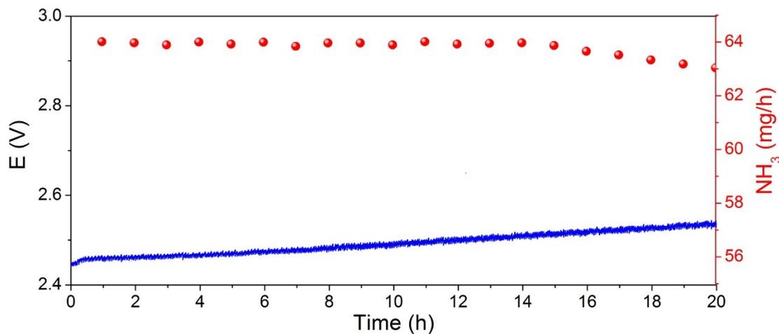
**Figure S24.** Stability test at a current density of 100 mA/cm<sup>2</sup> and the corresponding NH<sub>3</sub> yield rate at one hour interval in the PEM reactor.
