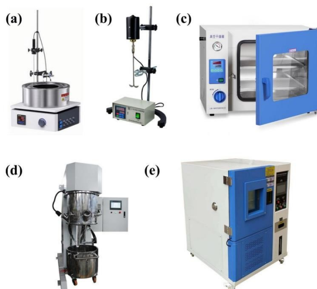
Figure S8. Oil bath pot (a), mechanical stirrer (b) and incubator (c) for laboratory; mechanical stirrer (d) and incubator (e) for industry.
