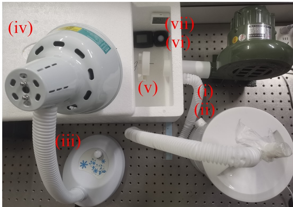
(i) Blower; (ii) Humidifier; (iii) Heating lamp; (iv) Foam insulation box; (v) Teng wind speed sensor; (vi) Illuminance sensor ;(vii) Temperature and humidity sensor
