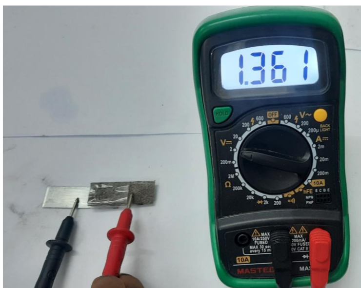
Fig. S27 Photograph displaying measured open-circuit-voltage of 1.361 V for solid state ZAB using PAM-h electrolyte for NiO/Ni-SACs/mNC1000.
