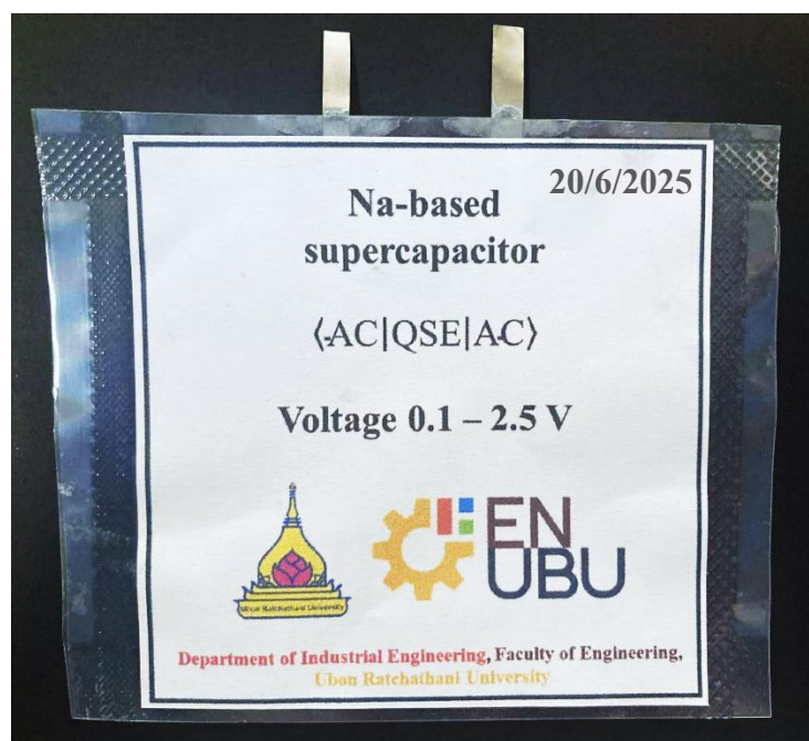
Figure S15. Photograph of the prepared pouch cell assembled between AC electrodes (square shapes of 1 \times 1 \text{ cm}^2 ) with an active mass material of approximately 2 \text{ mg/cm}^2 and the QSEs (thickness of 1 mm).
