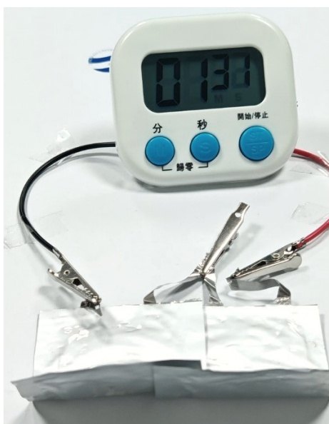
Fig. S23. Photograph of \text{MnO}_2||\text{Zn} pouch cell under bending states.
