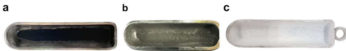
Figure S4. Photographs of quartz boats loaded with catalysts before and after synthesis. a) raw catalyst. b) BNNT. c) MgO-BN core/shell nanowires.
