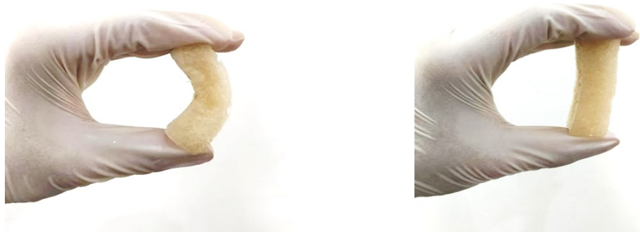
Fig. S8. Photograph of an elasticity test of hydrogel.
