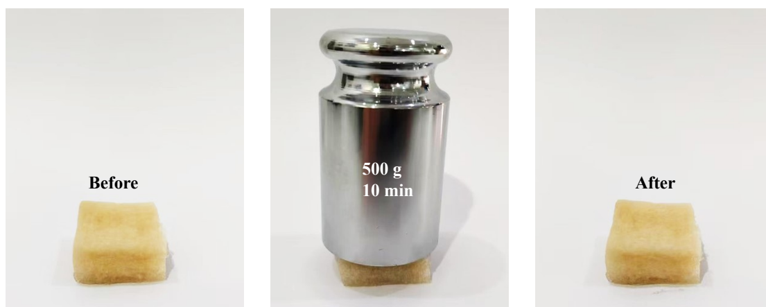
Fig. S9. Comparison of hydrogel before and after bearing a 500 g weight.
