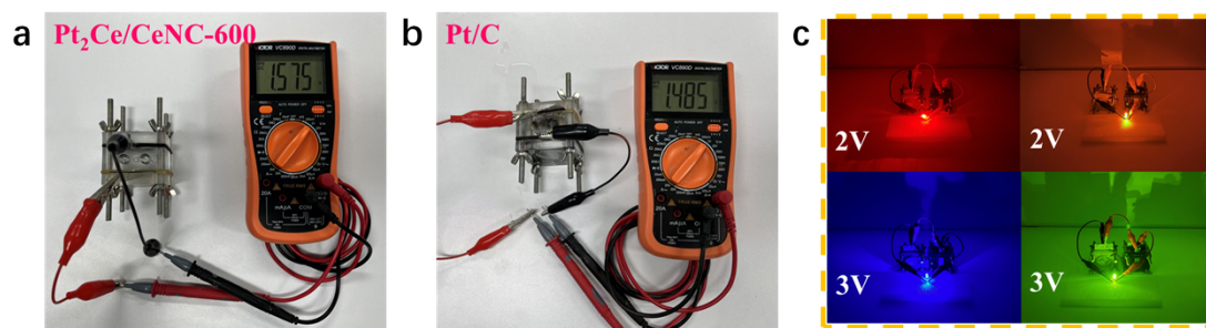
204 Figure S18. (a) Open-circuit voltage of Pt 2 Ce/CeNC-600. (b) Open- 205 circuit voltage of Pt/C. (c) Photograph of lighting a light-emitting diode 206 (2.0–3.0 V) by connecting two Pt 2 Ce/CeNC-600 based ZABs in series.
