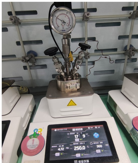
Figure S26 High-temperature and high-pressure reactor used for polyolefin hydrogenolysis reactions (Shanghai Yanzheng Experimental Instrument Co., Ltd.).
