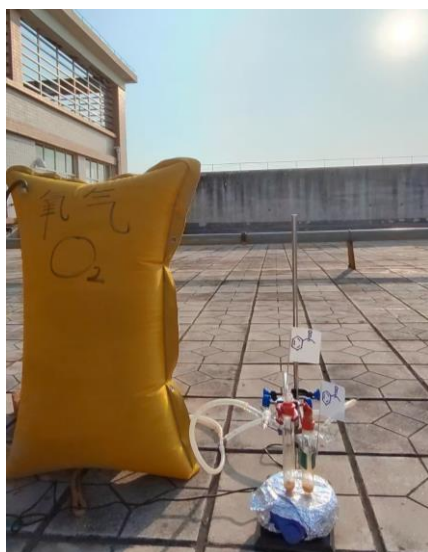
Figure S18. Experimental setup for photocatalytic oxidation of thioethers under outdoor
