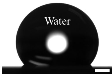
45 Figure S2. Image showing water droplet on a 0.45 \mu\text{m} PES membrane modified solely with Cl- 46 PDMS. Scale bar represents 500 \mu\text{m} .
