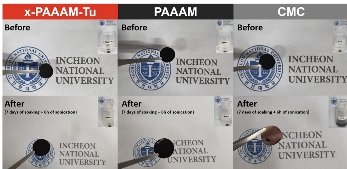
Fig S10. Digital photographs of the x-PAAAM-Tu, PAAAM, and CMC electrodes before (top) and after (bottom) soaking for 7 days and sonication for 6 hours.
