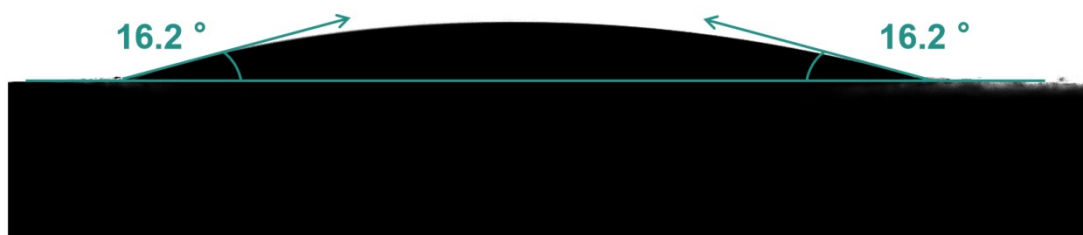
Figure S20. The measurement results of the water contact angle of Ac@[Ca-NDI] MOCF.
