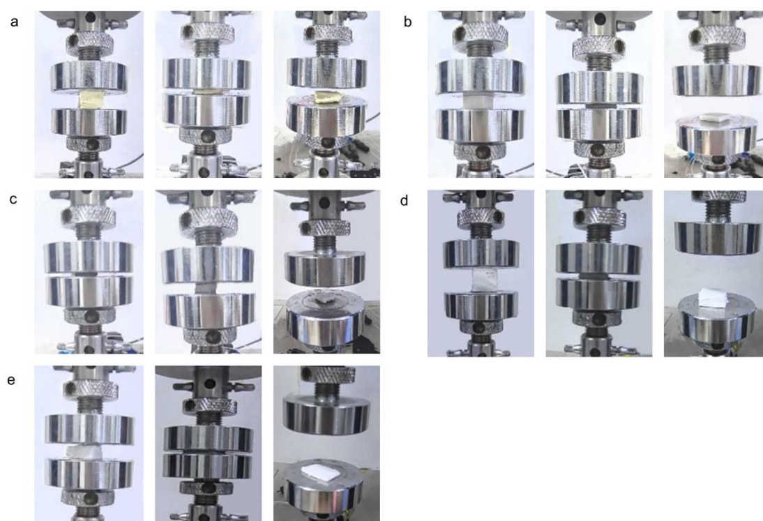
Fig. S26. Mechanical compression photos of (a) CS-A; (b) Gel-A; (c) PVA-A, (d) MC-A; (e) PAM-A.
