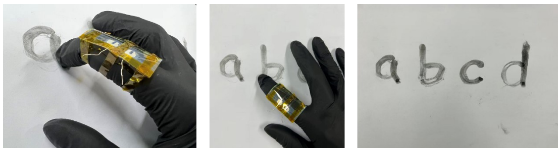
Figure S10. Photographs demonstrating the PITH device attached to a gloved finger during the handwriting of different letters.
