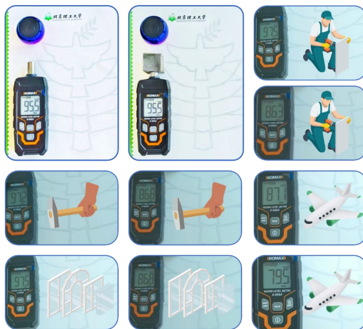
Figure S3. Ambient noise levels in simulated environments without FPUF-3: electric drilling, wall demolition, glass friction and aircraft engine operation.
