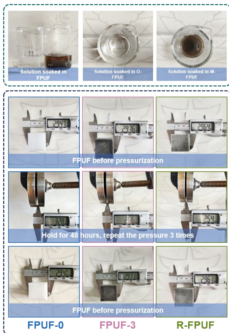
Figure S8. FPUF-3 recovery treatment and compression–recovery process of FPUF-0, FPUF-3 and R-FPUF under 90% strain.
