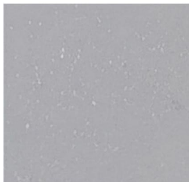
Supplementary Figure 5. The physical photo of the film after being dried in air for 48 hours. From the photo, it was clear that the film formed by this method was uneven and there was obvious precipitation.
