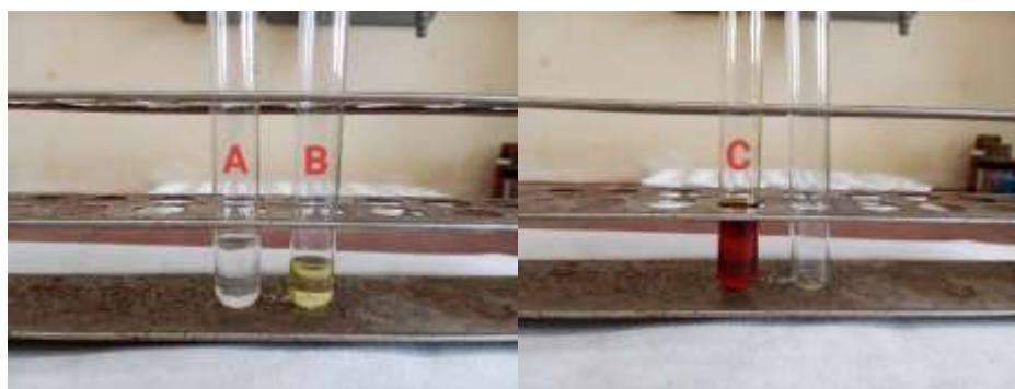
Figure S2. A) Commercially available \text{H}_2\text{O}_2 , B) KI-glacial acetic acid solution, and C) resulting solution after mixture of A and B ( positive result ).
