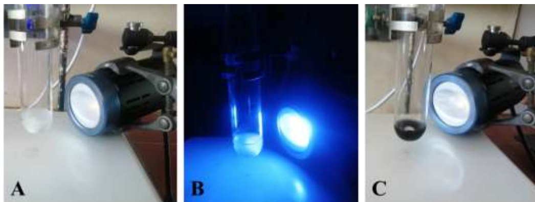
Figure S6. Setup utilized for the photochemical aerobic oxidation reaction (Blue LED, Kessil PR 160L, 456 nm). Reaction mixture before irradiation (A), during irradiation (B) and after completion of the reaction (C).
