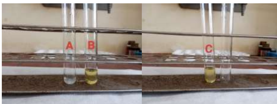
Figure S4. A) Non-irradiated reaction mixture, B) KI-glacial acetic acid solution, and C) resulting solution after mixture of A and B ( negative result ).
