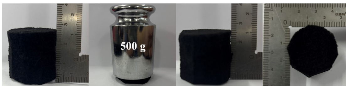
8 Fig. S1 Compression and recovery of the CuNPs@PANI-PPy/PVA-4.
