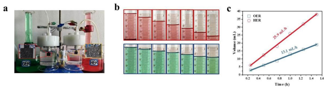
Figure S28. (a) Optical photograph of the assembled electrolyzer. (b) Photographs of \text{H}_2 and \text{O}_2 collected at different times. (c) The amount of \text{H}_2 and \text{O}_2 varying with time.
