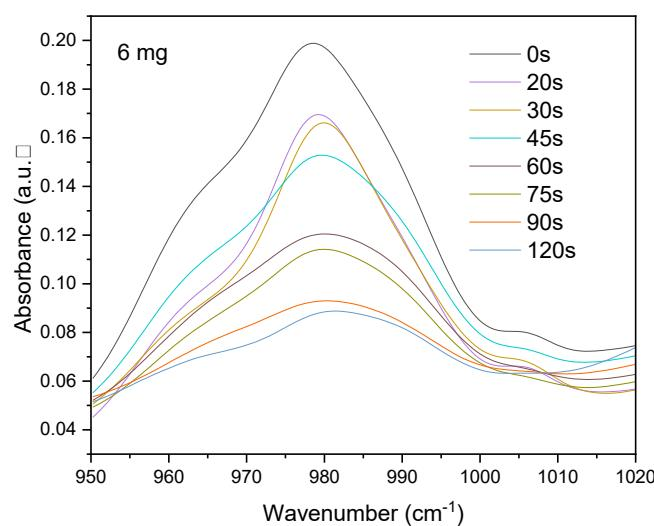
Figure S1. FTIR absorbance curves of 35AM65VP anhydrate gel with 6 mg curcumin after exposure of different times.
