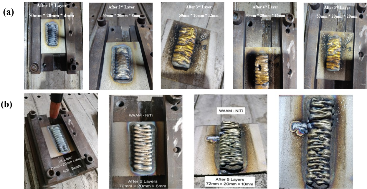
Figure S2. Layer-by-layer buildup of the nitinol for 3-D printing in (a) 2 nd trial, (b) 1 st trial
