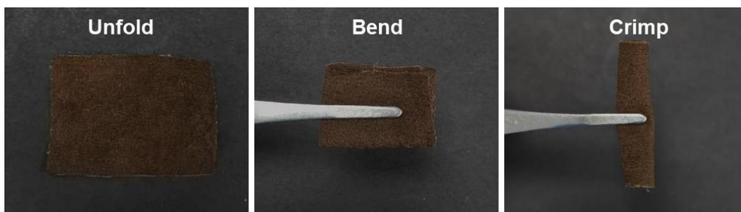
Fig. S3. Photos of SFM@PDA-RSF under unfold, bend and crimp.
