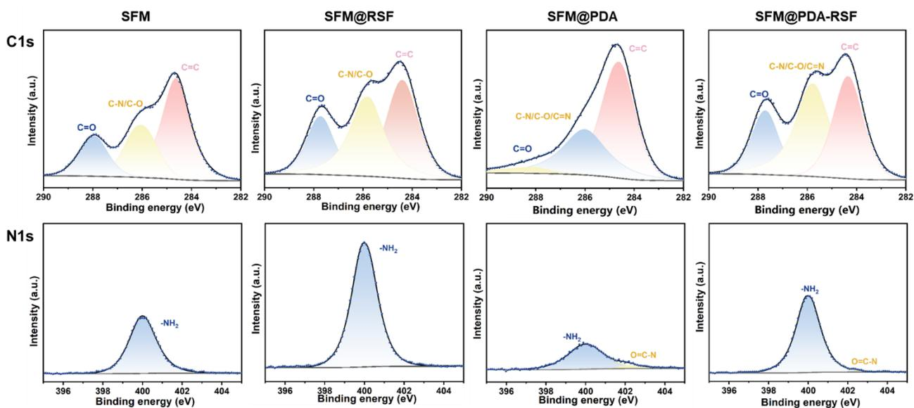
Fig. S2. High-resolution XPS spectra of C1s and N1s in different meshes.
