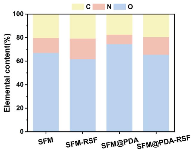
Fig. S1. The composition percentage of elements C, N and O in the xps spectrum.
