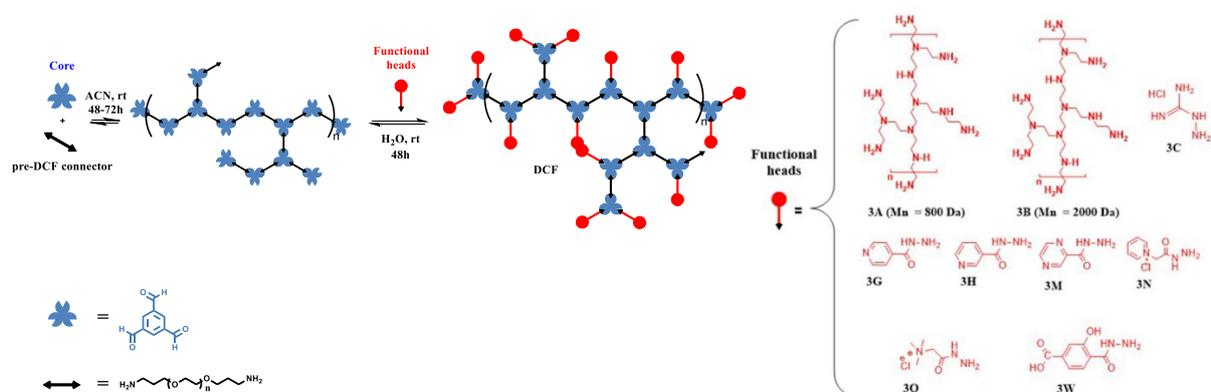
Figure S1. Representation of DCF Components and Preparation Procedure
