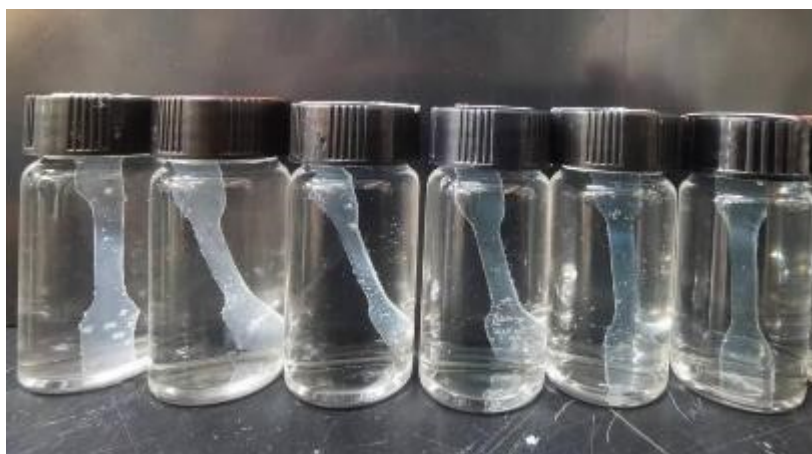
Fig.S19 State of W-P-DA 2 -x% films after immersion in water for 24 h (W-P-DA 2 -0%→5%, from the left to the right).
