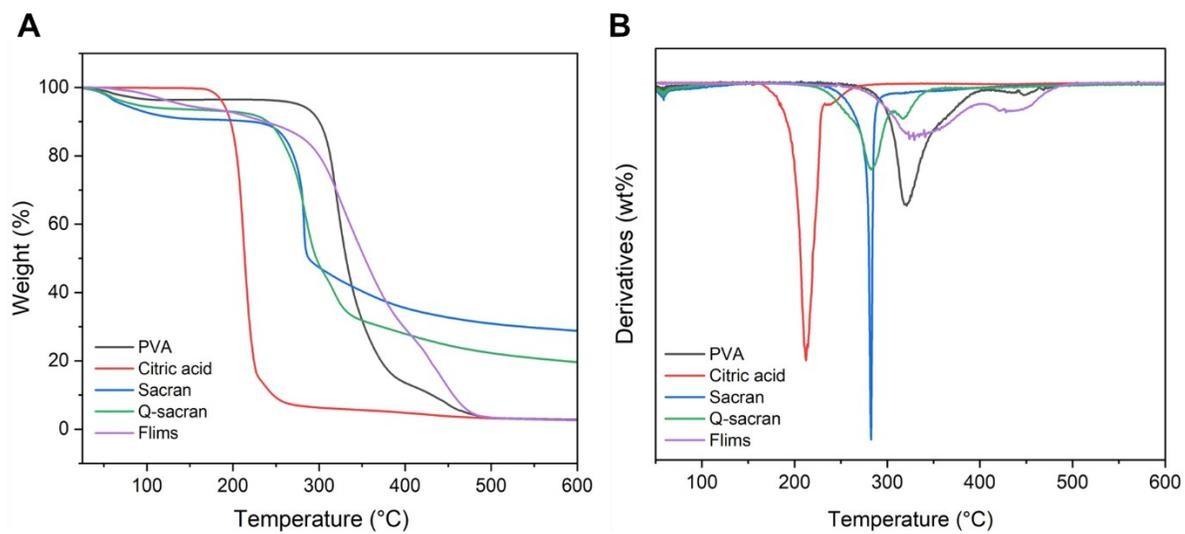
**Figure S3.** A) Thermogravimetric curves (TGA) of poly(vinyl alcohol) (PVA), citric acid (CA), sacran, quaternised-sacran, and film settings; B) derivative thermogravimetric (DTG) analysis curves.
