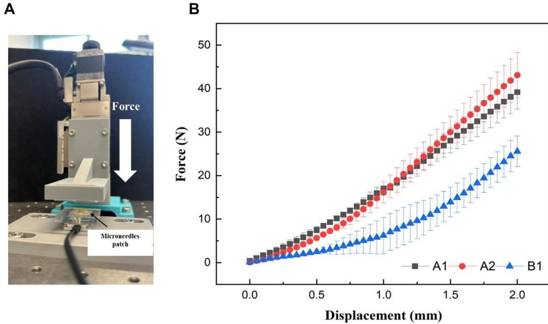
**Figure S1.** (A) Experimental set-up for mechanical testing of microneedle patches showing the direction of force application. (B) Force–displacement curves of different microneedle formulations (A1, A2, and B1) under compression testing. A1 and A2 demonstrate similar mechanical behaviour, with the maximum force of approximately 40 N at 2.0-mm displacement. B1 shows lower mechanical strength, with the maximum force of approximately 25 N. Data are presented as mean±SD.
