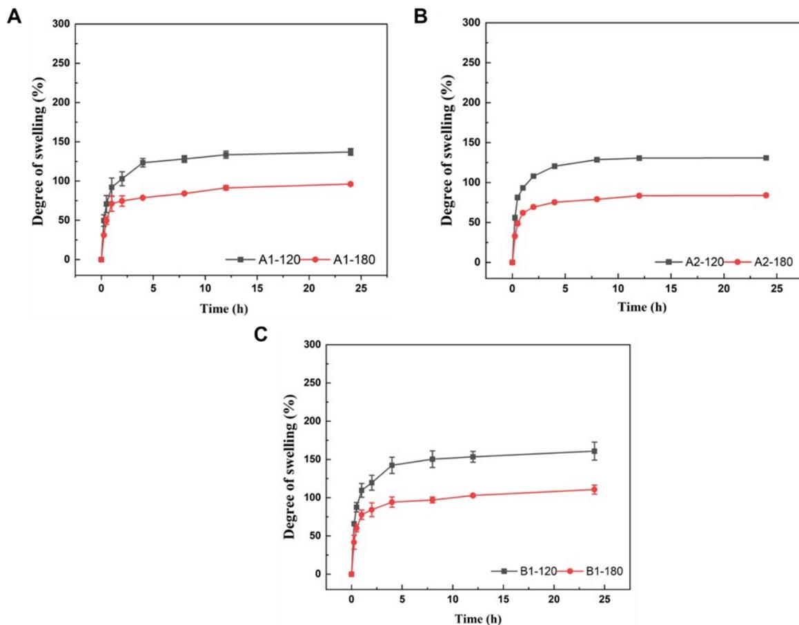
**Figure S2.** Degree of swelling in poly(vinyl alcohol) (PVA)/sacran hydrogel microneedles (HMNs) (A1 and A2) and PVA/Q-sacran (B1) with crosslinking durations of 120 and 180 min. The concentration of citric acid in the formulation was fixed at 1.0% w/v. All data are reported as mean  $\pm$  SD,  $n = 3$ .
