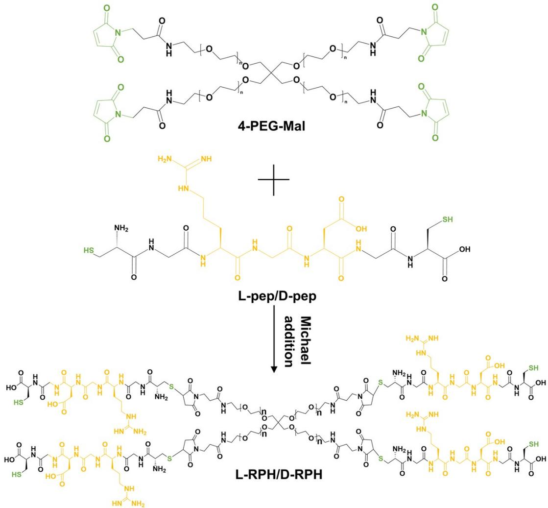
**Figure S1.** Schematic illustration of the reaction between peptides and 4-PEG-Mal forming a hydrogel via Michael addition.
