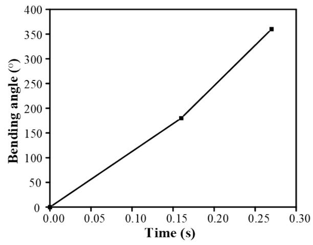
Figure S8. Time-dependent bending angle of the petal-type actuator.
