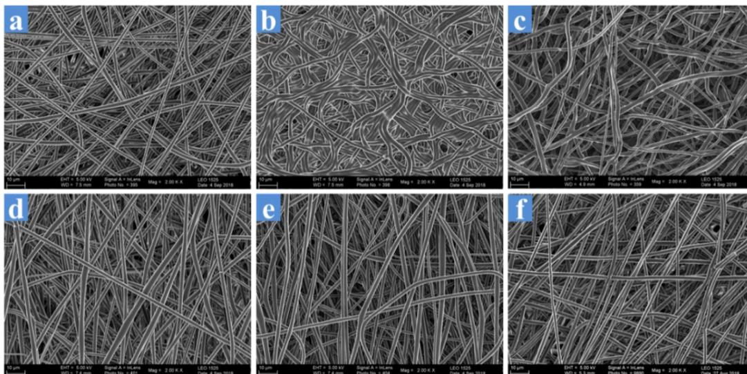
Figure S4. SEM images of the morphologies of nanofibers. (a) Crosslinked P(NIPAm-*co*-ABP) mixed AuNPs nanofibers; (b) after alternately immersing in water at 4 °C and (c) 40 °C for 1 min; (d) crosslinked P(GMA-*co*-ABP) nanofibers; (e) after alternately immersing in water at 4 °C and (f) 40 °C for 1 min.
