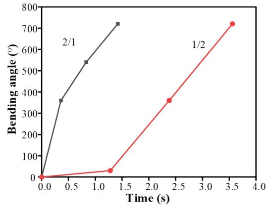
Figure S7. Time-dependent bending angle of actuator with different thickness ratio between the active layer and the passive layer .
