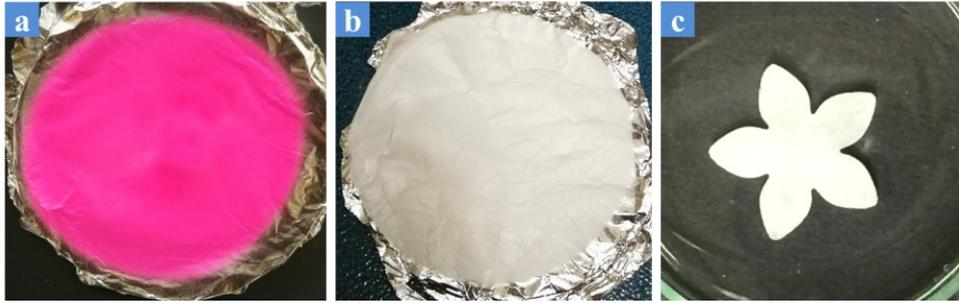
Figure S6. Photo of electrospun nanofiber membranes. (a) Passive layer fabricated from P(GMA-*co*-ABP) mixed with 0.3 wt% rhodamine B; (b) active layer spun from P(NIPAm-*co*-ABP); (c) petal-shaped bilayer actuator.
