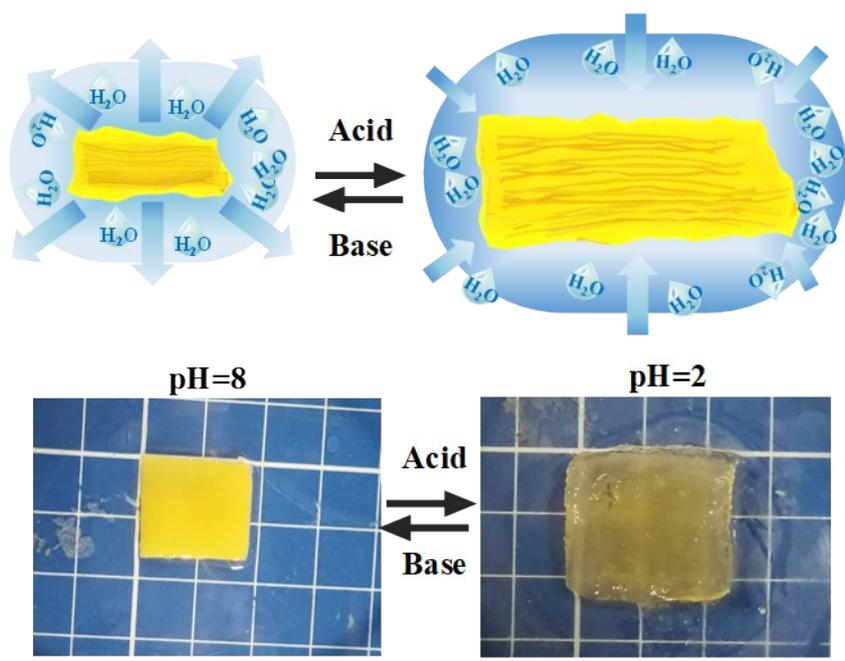
Figure S5. The scheme and photos of pH-responsive reversible deformation.
