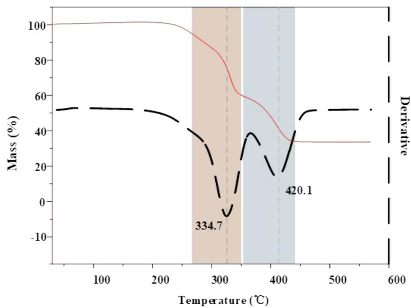
Figure S1. Thermal gravimetric analyzer curve of synthesized P(DEAEMA-*co*-MMA-*co*-ABP).
