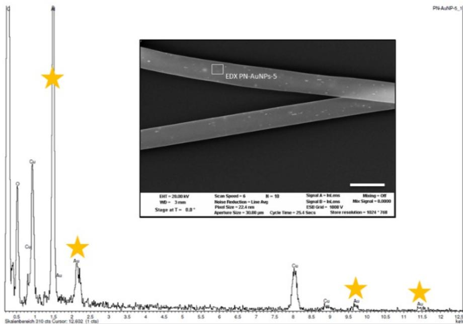
Figure S3. High-resolution SEM image of P(NIPAM-*co*-ABP) mixed AuNPs nanofibers (inserted image) and its corresponding EDX spectrum.
