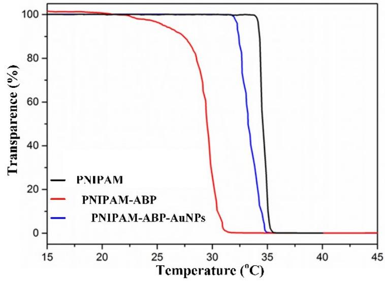
Figure S2. LCST curves of pure PNIPAM, copolymers P(NIPAM-*co*-ABP), and copolymers P(NIPAM-*co*-ABP) mixed with AuNPs.
