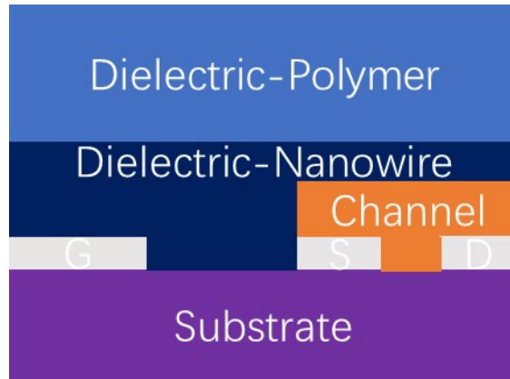
Figure S3 This coplanar gate highlights the complete cross-sectional view of the transistor, including the substrate, source(S)-drain(D) gate electrode(G), channel, and quasi-solid-state nanofiber composite electrolyte.
