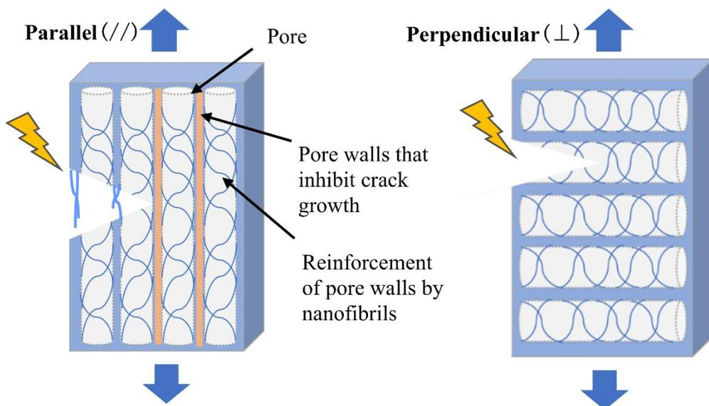
**Figure S9.** A schematic representation of the hierarchical structure of the PEDOT/DF-SO gel under elongation. When the hydrogel is stretched parallel (//) to the freezing direction, it resiliently withstands even when cracks occur. When the hydrogel is stretched perpendicular ( $\perp$ ) to the freezing direction, the fracture propagates along the pore walls.
