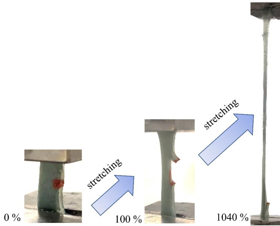
**Figure S10.** Photographic images during the tensile test with a 1 mm notch inserted.
