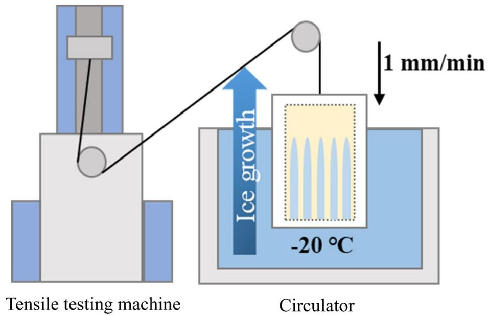
**Figure S1.** Schematic diagram of directional freezing device.
