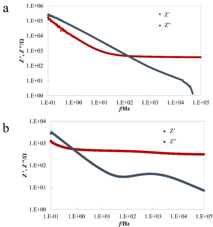
**Figure S12.** AC impedance spectra of (a) DF-SO gel and (b) PEDOT/DF-SO gel ( $f$ : frequency,  $Z'$ : real part,  $Z''$ : imaginary part).
