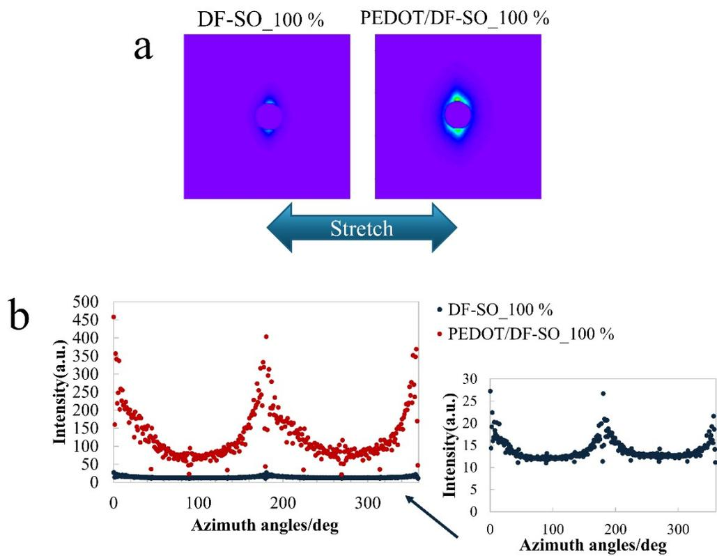
**Figure S13.** The SAXS results for DF-SO gel and PEDOT/DF-SO gel at 100 % elongation. (a) 2D scattering profiles and (b) azimuth distribution curve.
