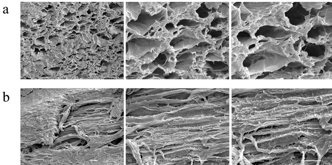
**Figure S5.** SEM images of hydrogels after salting-out, (a) cut perpendicular ( $\perp$ ) to the freezing direction and (b) cut parallel ( $\parallel$ ) to the freezing direction.
