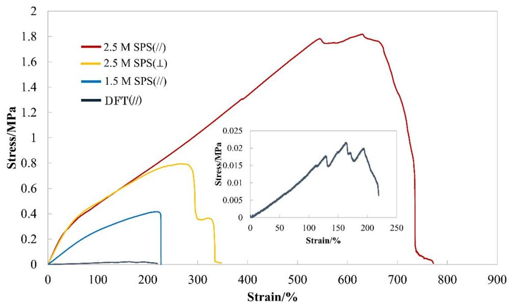
**Figure S8.** The results of the tensile tests for the DF-SO gels. In DF-SO gel (//), increasing the SPS concentration to the saturation point around 2.5 M improved the fracture strain of the resulting hydrogel (from  $378 \pm 137$  % at 1.5 M to  $855 \pm 96$  % at 2.5 M).
