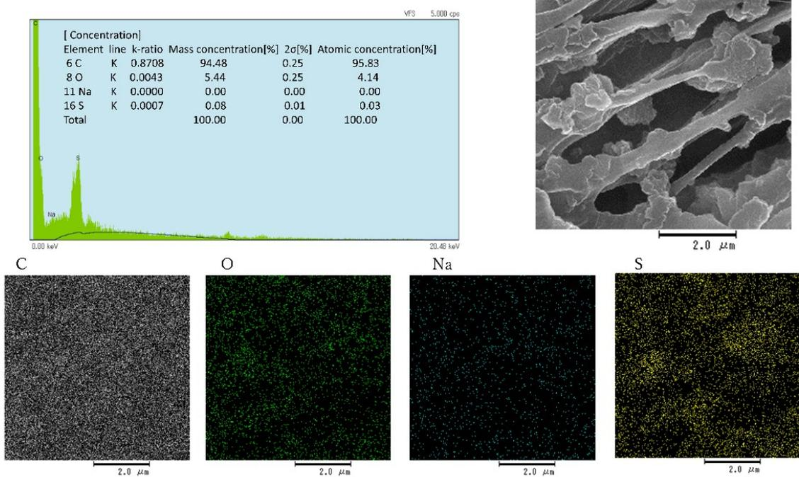
**Figure S7.** Elemental concentrations in the PEDOT/DF-SO gel were determined by energy-dispersive X-ray spectroscopy (EDX) analysis.
