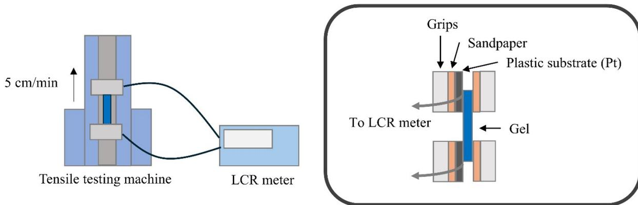
**Figure S2.** Schematic diagram of impedance measurement during elongation.
