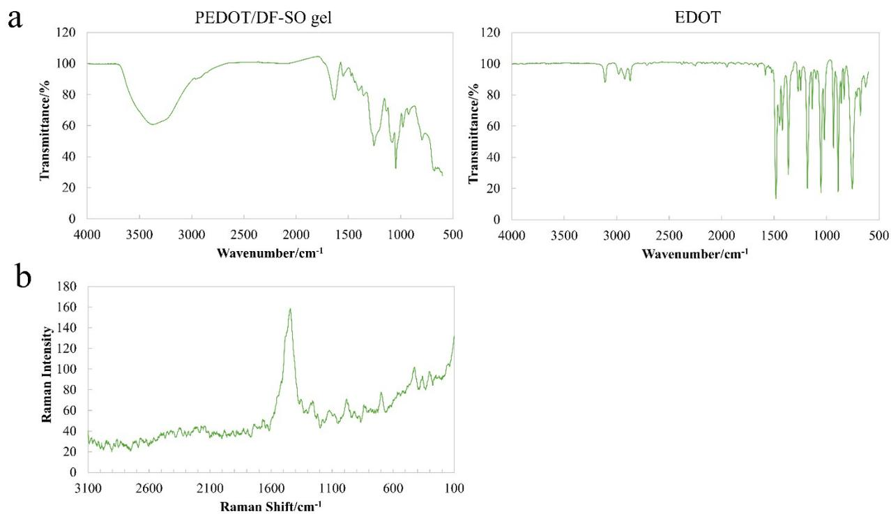
**Figure S6.** (a) Fourier-transform infrared (IR) spectroscopy with attenuated total reflection (ATR) of the PEDOT/DF-SO gel and EDOT. (b) Raman spectrum of the PEDOT/DF-SO gel.
