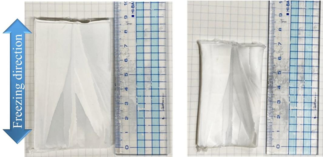
**Figure S4.** The frozen body of 10 % PVA aqueous solution after directional freezing: DF gel (left). The 10 % PVA hydrogel after salting-out phase separation with 2.5 M sodium persulfate aqueous solution: DF-SO gel (right).
